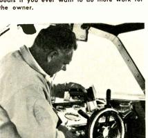
Black and Decker's battery-powered drill being used aboard boat to drill holes for new instrument installation.
