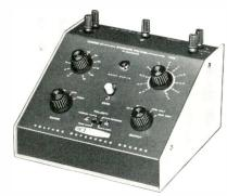
and research laboratories, is announced. Voltages produced by this instrument may be used for calibration of laboratory instruments or for accurate measurement of unknown voltages, it was said. Output voltage is variable from 0 to 100 v dc with readout made on three calibrated dials, COURSE VOLT-
