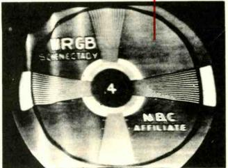
Lines caused by yoke trouble have a greater intensity at the top and bottom of the picture. Note that the raster lines are bent where white line crosses them. This is peculiar to yoke troubles.
