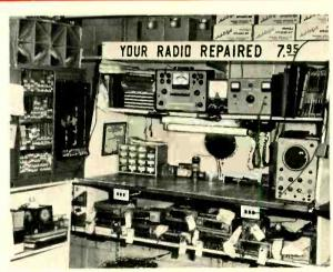
Fig. 3—Test and repair bench for auto radios is organized for maximum efficiency.
