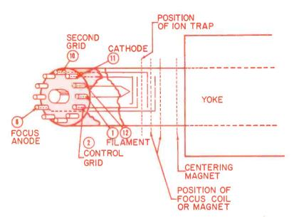
Fig. 1.—The physical relationship of the CRT's elements, the base and its accessories.
