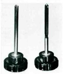
Knob reamers with handles made from old instrument knobs. At left is "home made" reamer: at right is commercially made fluted reamer.
