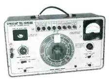
Sprague capacitor analyzer.
