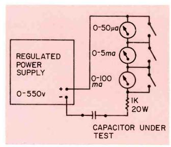
Fig. 1—Basic circuit used to measure electrolytic capacitor leakage current.
