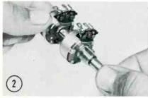
It's easy to assemble a dual concentric control (1). Components merely snap together (2). Courtesy Clarostat.
