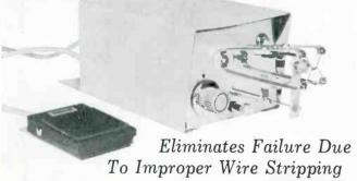
The new Sentry W-4 Thermal Wire Stripper is a foot switch, bench model especially designed for industrial wire stripping operations and will not nick, cut, stretch, or scrape the wire in any manner. Meets requirements of NASA specifications. It does not require adjusting for different sizes. Micrometer adjustment and rheostat temperature control.
