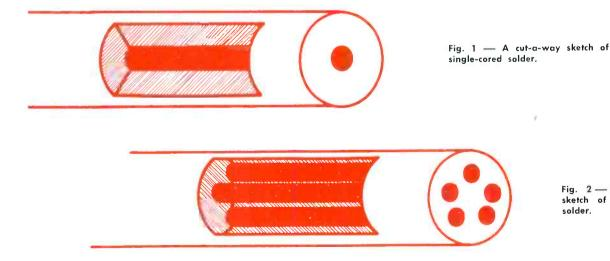
Fig. 2 — Cut-a-way sketch of a 5-core solder.
