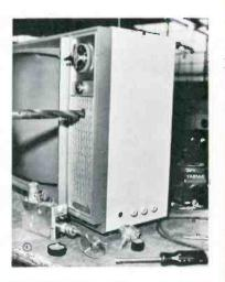
■ A UHF television converter kit that can be installed in about 45 minutes in consoles, table models, and most portables, has been developed. The converter tuner permits the TV dealer or service technician to customize television sets for his customers, make VHF television trade-ins more saleable, or replace defective UHF tuners. It tunes all channels, 14 through 83. The kit contains all necessary parts including tuner.
