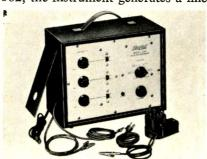
crosshatch pattern and the smallest dots available in anything but laboratory equipment, the maker said. A gated color-burst provides correct color alignment signals as well. Specifications indicated that the generator provides complete convergence signals — vertical bars, horizontal bars, crosshatch and dots —less than two lines wide and one line thick; a gun-killer for convergence and to facilitate purity adjustments; and a single-bar, crystalcontrolled color-burst signal. Hickok.
