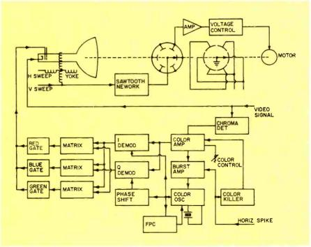
Block diagram of color converter showing points where signal is taken from standard TV.
