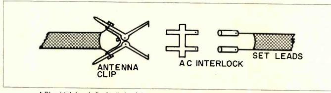
A TV ac interlock works fine for clipping clothes pin antenna connectors to short set leads when back is removed.
