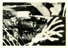
Ringing coil in dot generator circuit is adjusted for sharp, arrow "dots" while tuned to a strong signal.
