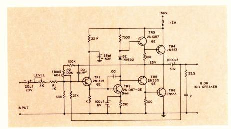
Fig. 1—Diagram of a transistorized audio amplifier.
