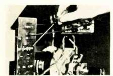
Terminal strip on rear of chassis is in series with filaments. When the link is opened, 13 amps are available to operate degaussing coil.
