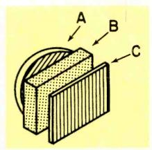
Fig. 1—Filter system shows rotating polariod (A), dispersion filter (B) and the stationary polariod filter (C).
