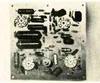
Sound-sync circuit board before installation on the chassis.
