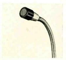
the use of unusually long cables without affecting response or level, it is said. Specifications gave frequency response as 40 to 10,000 cps with rising characteristic to 4500 cps; output level, -56.0 db (o db = 1 mw per 10 microbars); net weight: 5 oz. Price, \$32.50. Shure.
