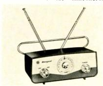
Models are also available without built-in antennas. All models are furniture styled in polystyrene cases in autumn brown trimmed with brushed gold and feature 3 gang capacitive tuning elements, 6DZ4 oscillator tube, isolated power supply with silicon rectifier, 1N82A diode and completely enclosed cabinets. Specifications indicate all models exceed FCC radiation requirements. Six models are priced from \$29.95 to \$69.95. Winegard.
