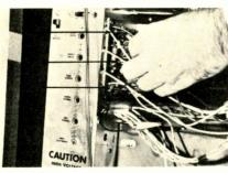
Two permanently installed clip leads are used to kill CRT guns. Three 100K resistors pointed out by arrows are test points.
