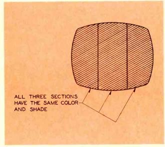
Fig. 2—Center area of screen will be the same brightness level as the two outside areas when the demodulator is adjusted properly.
