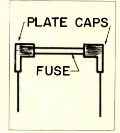
Salvaged tube grid-caps used to mount fuses above chassis.
