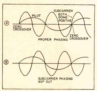
Fig. 5 (A)—Proper pilot frequency phasing. (B)—Proper subcarrier phasing.
