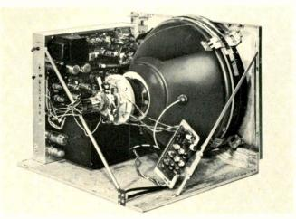
Rack mounted '63 model. Convergence controls are permanently mounted on brace as shown. The '64 models all employ the wall mount within the cabinet.
