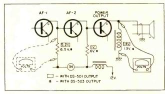
Delco auto radio transistor checks for dead radio.
