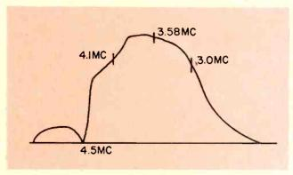
Fig. 3—Appearance of average color amplifier response curve.
