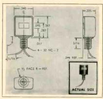
3K17, the head is especially designed for micro-miniature tape recording uses. The head is approx-
