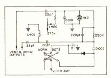
Circuit used in the built in dot generator is a simple neon oscillator triggered from horizontal and vertical pulses.
