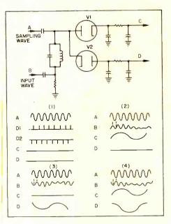
Fig. 1 — Functional diagram of two-diode sampler and waveform operation analysis.
