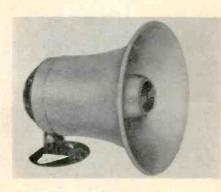
operation, the maker reported. Specifications rate the unit's power input at 6 w and frequency response from 400 to 13,000 cps. Bell diameter 7½ in., overall depth 6-3/8 in. Price \$25.25. Atlas Sound.
