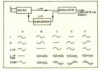
Fig. 2-Make-up of composite FM signal.
