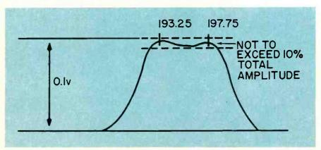
Fig. 1—Channel 10 RF response curve at the channel selector output.
