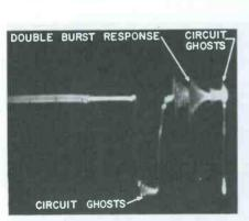
Fig. 6 — We must use a low-Q colorsubcarrier trap to eliminate circuit ghosts and double bursts,
