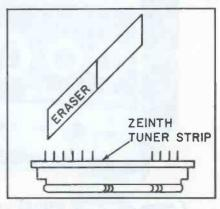
Eraser cleans contact strips on pin type tuner strips.
