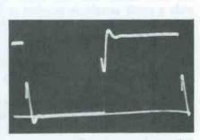
Fig. 5 — A low-Q wavemeter gives a ringing pattern which is damped and dies out quickly. It gives information about the leading edge only.
