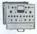
Triplett's tube analyzer is a lab-type mutual conductance instrument. The unit can also be used to plot characteristic curves, \$349.50.
