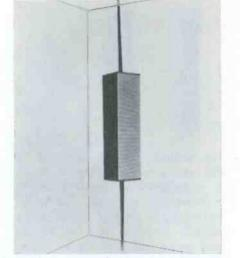
all four sides for use as a room divider. Internal capacity is in excess of 4620 cu in. and acoustic lining is employed to prevent bass reverberation. Enclosures are supplied with Jensen 8 in. extended range woofer, 31/2 in. tweeter, and precision cross-over network. Dimensions of the enclosure are 40 in. high x 11 in. wide x  $10\frac{1}{4}$  in. deep. Designated Model SM8-C the complete unit lists for \$66.90. Wald, Inc.
