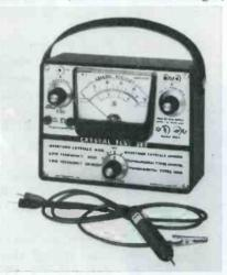
audio output across voice coil, and beat note in RF comparisons. It will generate a crystal controlled RF signal with 400 cps tone modulation and will serve as a 0.05 v audio frequency signal source. It retails for \$48.95 net. Seco Electronics Inc.
