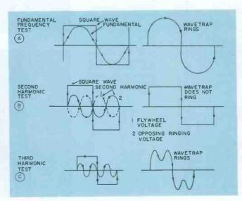
Fig. 7 (A) — Fundamental ringing frequency is sustained on each half cycle because the square wave and the ringing sinewave are always in same direction. (B) - A second-harmonic ringing frequency cannot be developed by the wave trap. A second harmonic of opposing phases is associated with the leading and trailing edges. (C) A third-harmonic ringing is sustained on each half-cycle of the squarewave.
