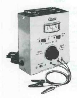
E l e c t r o Products Laboratories EC-3 Power Supply at \$19.95 — Small power supplies have become an important part of servicing transistor equipment. Some of the features of the EC-3 are particularly interesting: The bias is continuously variable from 0 to 7 v; the supply voltage is continuously variable from 0 to 20 v; the maximum rated voltage output can supply 150 ma continuously; and both bias supply voltages and ma are read on the same meter.
