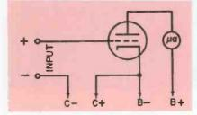
Fig. 1 — Fundamental VTVM circuit.
