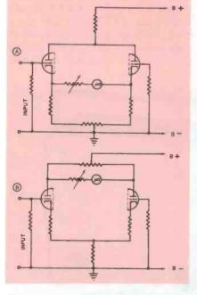
Fig. 3 (A) — Degenerative cathode-series VTVM bridge circuit. (B) — Push-pull dc amplifier bridge.
