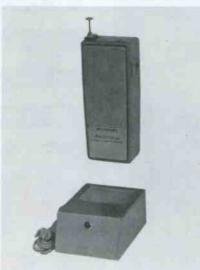
uses a 117 vac power supply converter to run on house current. Special features of the TRC-2 include push-to-talk operation, alltransistor operation with 9 transistors and 1 diode, long-short range control for sharp reception at every distance, small size (only  $6^{1/4} \times 2^{3/8} \times 1^{5/8}$  in.) and lightweight (about 2 lb). The TRC-2 sells for \$39.95. The ac/dc power supply converter, with special plug-in receptable sells for \$6.95. Radio Shack Corp.
