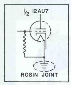
Rosin joint on video tube socket caused ac to be impressed on grid.
