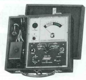
Mercury's Model 800 tester-reactivator.
