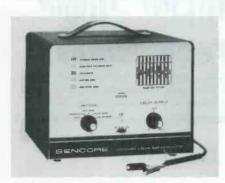
dialing any of the five patterns. Signal output is adequate to over-ride most local channels. Other low channels can be selected if desired by simple slug adjustment in rear. Stability is said to be insured by crystal controlled circuits, factory pre-aged vacuum tubes and standby position on the on-off switch. The CG126 weighs less than 10 lb. and measures only 11 x 8 x 6 in. providing portability for home or shop service. The CG126 color bar dot generator sells for \$99.50. Sencore.
