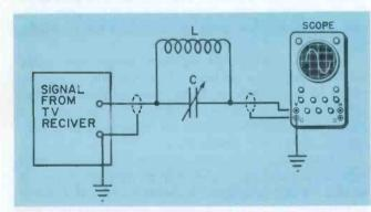
Fig. 2 — A hookup using a simple wavemeter or calibrated trap circuit will reveal harmonics of a complex waveform on the scope.
