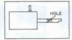
Fiber glass pin prevents slippage on insulated tuner shafts.
