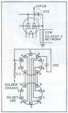
Top — Bypassing faulty capacitor in Philico chassis can be accomplished without chassis removal. Cutting marked lead No. 1 on network No. 30-6507-2, above the chassis. This lead is easily reached by pulling the 5U4 removes 2.2  $\mu$  resistor from network. Bottom — Wiring of new circuit.
