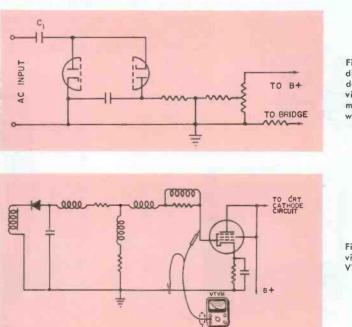
Fig. 4 — Doublediode VTVM voltage doubler ac input provides P-P measurements for complex waveforms.
