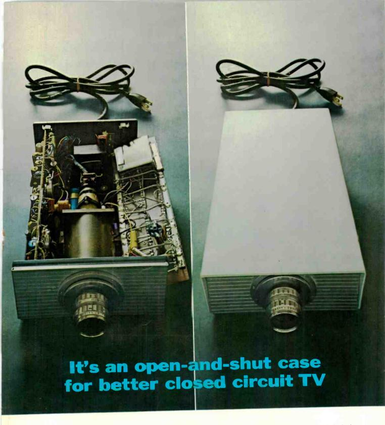
Consider the Norelco Television Camera. Open, it exposes its secrets of ruggedness and long life: no tubes to burn out—just tough little transistors...pivoted side panels for easy inspection and repair in the remote event of a malfunction...room to accommodate the larger Plumicon tube, when available.
