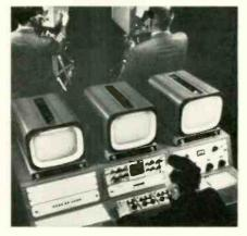
switched to the mixer output bus. The audio level of any one of 11 signals is through a master gain control and is monitored by a VU meter. ETV Sales, General Electric Co.
