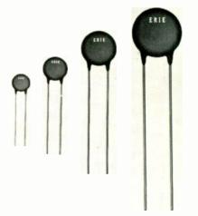
Capacitors to 0.47 µf, 25 vdcw, is offered in the "Transcap" line of ceramic capacitors. A new style offers 0.22  $\mu$ f in a case size of only 0.895 in. x 0.156 in. thick and  $0.47 \ \mu f$ in a case size of only 0.895 in. dia x 0.200 in. thick. Besides a very high capacitance per unit volume, another advantage cited for these capacitors is that the high resistivity
