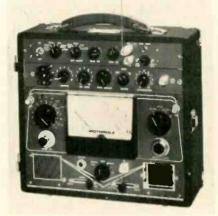
Motorola's two-way mobile test set, S-1059A, has built-in transistorized deviation meter.
