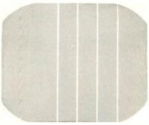
Damper tube or yoke are most frequently at fault when light wrinkles appear in raster.
