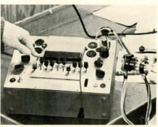
Completed tester with rectifier tube plugged into the spare socket. The adapter cable is attached in the same manner as for CRT testing.
