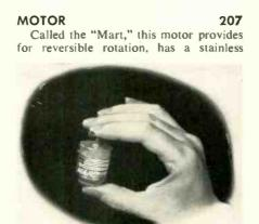
steel shaft, graphite brushes and sintered magnets and is designed to deliver up to 500 hr of service, continuous duty, at full load, according to the manufacturers. No-load speed is 7500 RPM operating load speed 5000 RPM and the motor produces a minimum of 0.125 oz in. of torque under operating load. Operating voltage may vary from 1.25 to 24 v and amp input is 0.75 (at 3 v) under operating load. Martronics, Inc. and up to 220 Mc on second harmonic.
