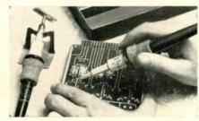
Low wattage iron equipped with slotted desoldering tip may be used to remove capacitor from printed circuit board. Iron at left is equipped with bar type desoldering tip.
