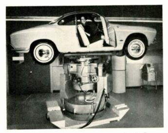
A 2000 lb sports car and its attractive passenger literally floats on air to demonstrate the load capacity of a precision air bearing servorate turntable. A similar type, designed and built by Dunn Engineering Corp., will test the inertial guidance system of the Saturn rocket. The turntable rotor rests on a thin film of compressed air, instead of the conventional ball or roller bearings.
