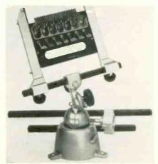
down for greatest accessibility for the work at hand. Model 315 PC board holder (complete with 10 in. holder arms. \$12.95. Wt. 1 lb. Colbert Die Cast Co.
