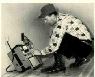
Technician uses Jerrold's Model 704B field strength meter to measure TV signal at a master distribution outlet.
