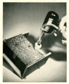
Oneida's desoldering attachment for guns can lift solder into a porcelain bowl when bulb is squeezed a few times.
