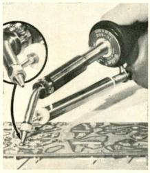
ENDECO's desoldering and resoldering iron removes molten solder by vacuum pickup.
