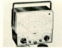
VTVM made by Triplett. Frequency response of this instrument can be extended to 250 mc with a special probe.
