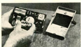
By turning the rheostat till the radio stops operating, the cut-off point can be measured with the voltmeter.
