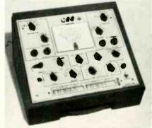
ranges cover from 0-0.5  $\mu$ a full scale to 0-25 ma full scale. A chopper and high-gain amplifier aid in leakage current measurement on the low-current scales. R D Instruments Div. Hickok Electrical Instrument Co.
