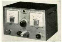
0-15 volts d-c at up to 3 amps. Designed for continuous duty, output is regulated to remain within .1% of indicated voltage with input varying from 105 to 125 volts. Filter circuitry is full wave, series shunt regulated, with 4 power transistors. Ripple factor is 10 mv RMS at 50% load, and 30 mv RMS at full load. All components are short circuit protected. Weight, 51/4 lbs. Size, 83% in. x 63% in. x 53% in. \$89.50. George Harmon Co., Inc.
