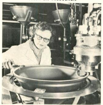
Solder application machine helps accelerate production of color CRT's at RCA's \$10 million Lancaster, Pa. plant, where \$1.5 million expansion program is underway to meet anticipated 250% increase in 1962 demand. The machine spreads a thin ribbon of special glass-sealing solder to the edge of a 21-inch type CRT envelope while it is rotating.
