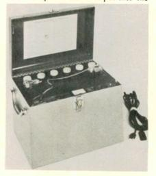
battery over the charging circuit. The recommended battery has a 55 amphour rating and is capable of storing approximately 660 watt-hours of energy. Of this, about 560 watt-hours are available at usable terminal voltage. Specifications include: output power, 140 watts max. continuous at 70-100% power factor, and 175 watts intermitent at 80-100% power factor for not over 15 minutes at 25% duty cycle. Cornell-Dubilier Electronics Div., Federal Pacific Electric Co., Fuquay Springs, N. Car.
