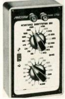
Model 1720 resistance substitution box permits direct substitution of 36 different resistance values through the use of either of two clearly marked rotary switches. Standard EIA resistance values in this unit range from 15 ohms to 10 megohms. Wattage dissipation of all resis-
