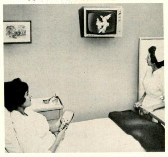
Designed especially for hospital lease plan, a 19" Sylvania TV set is equipped with combination remote control and a pillow speaker. Operates only when remote unit is plugged into an outlet adjacent to the patient's bed to give the hospital control over set operation. Has volume limiter and audio switch. Mounting of receiver on wall is on a special swivel bracket.
