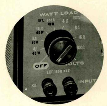
EICO's a-c/volt-wattmeter features watt load-compensation. Volts are calibrated in rms.
