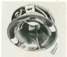
ment for four Westinghouse vokes. It is supplied already wired with the network components, and replaces Westinghouse parts 490V006H01 and H02, 490V006M01 and 490V007H01 in 29 chassis and 175 models. Horizontal coil inductance, 18.5 mh. Vertical inductance, 34 mh. Horizontal coil resistance, 33 ohms. Vertical resistance, 34 ohms. Stancor Electronics, 3501 W. Addison St., Chicago 18,
