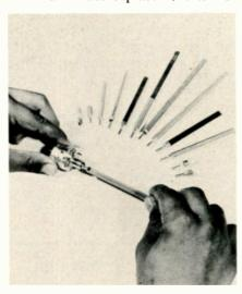
Clarostat control and a selection of precut shafts of various lengths.
