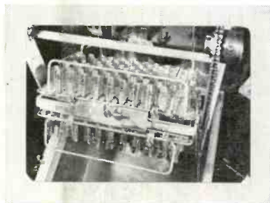
Guns emerging from ultrasonic cleaning tank. Still in the same tray, they are placed immediately in the radiant drying oven shown in the photograph at right.
