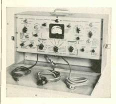
restores brightness by cathode sweeping, brings up old tubes by grid expansion, burns off low resistance K-G shorts, burns off high resistance interelement shorts, and welds open cathode tabs. \$189.50. Tele-Tronics Co., Ambler, Pa.
