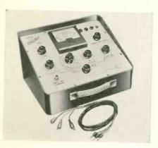
bridge, the total impedance is nulled. This all-transistorized tester measures the following in-circuit parameters: a-c Beta,  $I_e$ , transistor input resistance and base-emitter circuit impedance. Will also measure a-c Beta,  $I_e$ , and  $I_{cbe}$  out of circuit. \$129.50. Hickok Electrical Instrument Co., 10514 Dupont Ave., Cleveland 8, Ohio. For more data, circle 3-68-3 on coupon, p. 54
