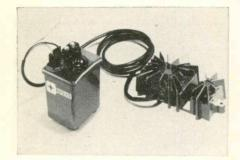
Fig. 1—Electric Autolite's transistorized ignition system, showing HV transformer, heotsinked transistor, and diade.
