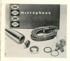
meet particular requirements. The microphone is designed around a special ceramic element which develops unusually high output and is unaffected by heat or moisture. Sensitivity, 1000 cps 52 db below 1v/microbar. Recommended load, 5 megohms. Frequency response, 30-10,000 cps. CBS Electronics, Danvers, Mass. For more data, circle 3-52-2 on coupon, p. 54
