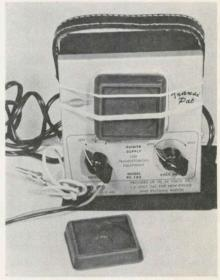
Fig. 2—Test instrument's meter face is protected by a rubber caster held in place by rubber bands.
