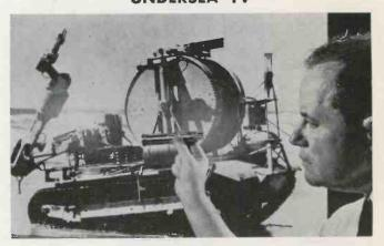
With this RCA vidicon tube, the Navy's new tank-like vehicle (in background) can see as it crawls along the ocean floor. Signals from the nautical TV cameras are transmitted to a land station via a special cable from the large reel. The vehicle is called RUM for Remote Underwater Manipulator. It was developed by U. of Cal.
