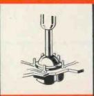
Cup Shaped De-Soldering Tiplet removes solder from circular multi-lug components in one
