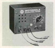
age, drift and other important characteristics. The test set performs its function by means of a simple audible indication. Current is drawn from the test set only during the actual test of a transistor. Motorola Inc., 4545 W. Augusta Blvd., Chicago 51, Ill.
