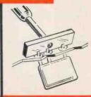
Bar Tiplet simultaneously melts solder on all multiple straight line network components.
