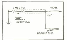
Fig. 10—Audio source for signal injection troubleshooting when audio generator is not available. The 2 meg pot adjusts gain.
