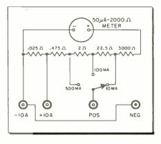
Fig. 1—Basic arrangement of shunt resistors in a VOM for d-c current measurements ranging from 10 ma to 10 amperes.
