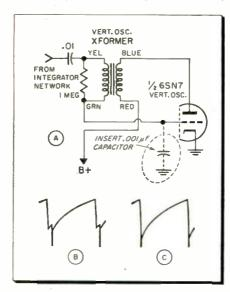
Fig. 1 (A)—Vertical jitter was eliminated by installing a .001 #f capacitor. (B)—distorted sync in waveform taken at the vertical oscillator plate of Ambassador TV. (C)—Normal waveform after installing capacitor.
