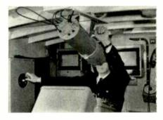
Fig. 4—Small-craft type radar unit shown mounted to bulkhead in the wheel-house.
