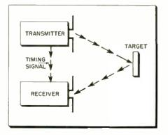
radar's master oscillator. Both trigger pulses for timing the r-f oscillator firing with the rest of the system, and in some sets, a gating pulse to instantly turn the receiver on after transmitter firing are provided by this unit.
