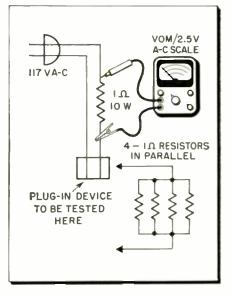
Fig. 6—Extension cord used for measuring power loads by employing a VOM's 2.5 a-c scale. By substituting four 1 ohm resistors, in parallel, currents up to 10 amperes can be measured on this scale.
