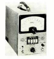
200,000 cps in four ranges. Accuracy is 3% or 1 cycle, whichever is greater. Output voltage: sine wave, 0 to 5.0 rms volts; square wave, 20 mv to 7.0 p-p volts \$129.95. Jackson Electrical Instrument Co., 124 McDonough St., Dayton, Ohio.
