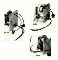
310 replaces Emerson 738142 and HO-311 replaces Emerson 738155. These exact replacements are used in 141 Emerson models and chassis without any circuit or chassis alteration. Chicago Standard Transformer Corp., 3501 Addison St., Chicago 18, Ill.
