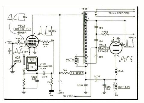
Fig. 3—Minimum milliammeter reading is desirable when a horizontal linearity coil is adjusted. Improper adjustment may overheat the flyback transformer due to excessive current.
