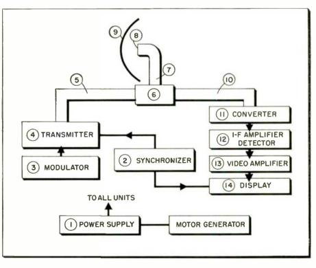
area under observation in a 360 degree pattern. The waves are reflected in all directions by any object they strike.
