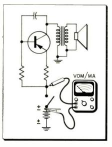
Fig. 4—Current overload in a transistor radio can be detected by inserting a VOM's milliamp scale in series with its load.
