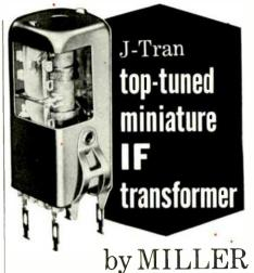
You can align both tuned circuits from the top of the shield. Unit is designed with tuning cores which have hex holes extending the length of the core. This construction permits aligning tool to pass through one core and engage the other.
