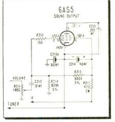
Fig. 2—Leaky coupling condenser to audio output grid caused channels 7 and 10 to fade out when volume control was varied.
