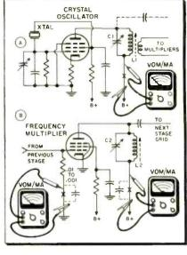
Fig. 7—All r-f stages of a radio transmitter can be accurately tuned to resonance with the oscillator's frequency by adjusting for maximum current reading in grid and minimum current reading in plate circuits.
