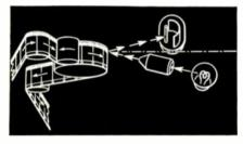
Fig. 2—Basic optical sound operation: light is focused on film's sound track; modulated light passing through film is reflected to a photoelectric cell.
