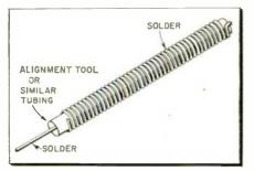
Fig. 3—Made from a length of hollow tubing, this handy solder dispenser is used like a pencil—eliminating a spool or loose coil.
