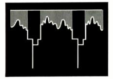
Fig. 2—Composite video waveform taken from the video detector at vertical frequency shows narrow, excessively peaked sync pulse spike, indicating open agc filter capacitor.
