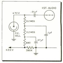
Fig. 9—This photoelectric cell loading circuit shows thorough decoupling of the voltage supply. Slight variations, such as coupling impedance combinations and adjustable resistors to vary the PE potential, are also encountered.
