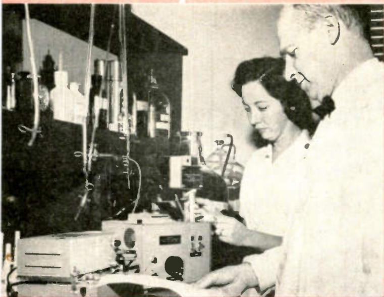
In Providence Hospital, Washington D.C., a research project for the identification of pathological conditions through serum protein analysis employs an American Instrument photorefractometer. The instrument passes light through the sample, scanning and recording the density. Routinely, the device aids multiple sclerosis diagnosis through gamma globulin analysis.
