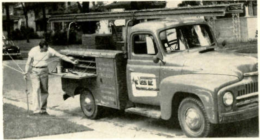
Fig. 1—Installation vehicles usually include a ladder as standard equipment. A magnesium or aluminum type offers easy maneuverability because of its light weight.
