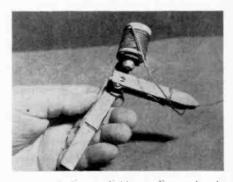
Fig. 3—Clothespin holder makes a handy solder dispenser and serves as "3rd hand."
