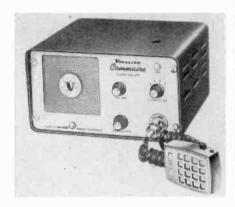
nel class D citizens band. It features the same audio circuitry as the ED-27, and has an improved transmitter. The receiver is a crystal-controlled double-conversion superheterodyne with a selectivity of 5 kc at points 6 db down and a sensitivity of  $\pm 0.3$  mv. \$189.50. Vocaline Co. of America, Old Saybrook, Conn. (ELECTRONIC TECHNICIAN 4-5)
