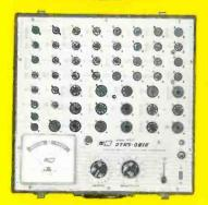
MODEL 650. Fastest and most complete portable Tube and Transistor Tester. Checks over 99% of the tubes most widely used in television receivers. Tests each section of multiple tubes separately for Gm, Shorts, Grid Emission, Gas, and Life. Includes spare sockets and filament voltages for future new tube types.
