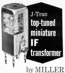
You can align both tuned circuits from the top of the shield. Unit is designed with tuning cores which have hex holes extending the length of the core. This construction permits aligning tool to pass through one core and engage the other.
