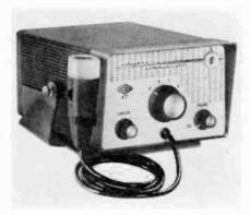
het receiver with r-f stage has automatic noise limiter and adjustable squelch for muted standby. Transmitter rating: 5 watts power input. Price, complete with press-to-talk microphone and crystals for one channel, \$149.95. Gonset Div., Young Spring & Wire Corp., 801 S. Main St., Burbank, Calif. (ELECTRONIC TECHNICIAN 1-5)
