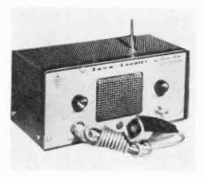
circuit minimum measurements of 3.25 watts over a 50 ohm non-inductive load; press-to-talk operation; and automatic squelch. Price, complete with %th wave whips, microphones, crystals, and printed forms and brochures, \$159.50. Utica Communications Corp., 19 S. La-Salle St., Chicago 3, Ill. (ELECTRONIC TECHNICIAN 1-7)
