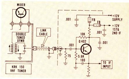
Fig. 1--Schematic of the IF emitter follower circuit employed in RCA's KCS176 and KCS177 chassis.
