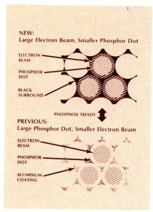
Fig. 4--Zenith's Chromacolor picture tube employs smaller color phosphors and surrounds them with jet-black material which absorbs ambient room light to improve contrast.
