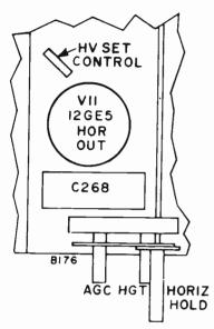
to the high voltage transformer. This power is controlled by the horizontal output tube plate current, which, in turn, is controlled by the horizontal output tube control grid bias voltage.
