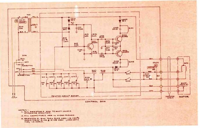
Fig. 3--Schematic diagram of the Cornell-Dubilier Model AR33 automatic rotator.
