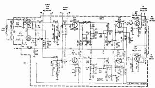
ratio and improve reliability by using smaller valued coupling capacitors. The high supply voltage for the amplifiers, +25v for the source leads and -32v for the drains (57v total). This supplies a high degree of self-bias for each stage through the bias resistors R17 and R35. With such a large self-bias voltage, consistent class "A" operation is realized over a wide tolerance range of J-FETs.
