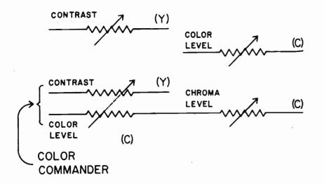
Fig. 6--The color Commander control employed in Zenith's 12A12C52 chassis permits color level tracking with contrast level by using a ganged CONTRAST and COLOR LEVEL control.
