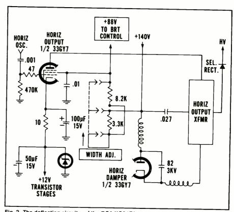
Fig. 2--The deflection circuitry of the RCA KCS176 and KCS177 chassis is similar with minor component changes to drive the large or small CRT. The basic circuitry is similar to the KCS169 chassis.
