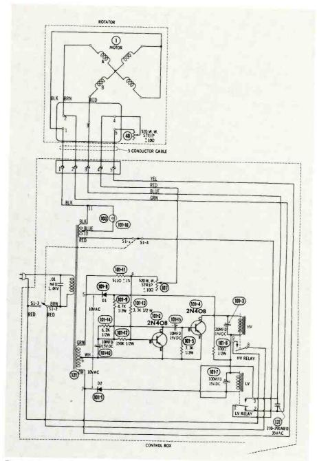
Fig. 1--Schematic diagram of the Alliance C-225 rotator system.
