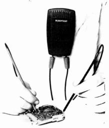
in a wide variety of production, maintenance and laboratory activities. Confirmation of a circuit continuity is obtained by an audible tone generated by a sonic signal generator. The unit as an indicator provides a low energy level through the circuit under test.
