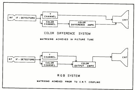
Fig. 5—A block diagram showing a simplified comparison between Zenith's RGB system and the previous color difference systems.
