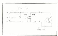
Simplified diagram of the dc beta circuit.
