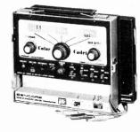
drain if the unit is accidentally left on. The unit is housed in vinyl-clad steel with brushed aluminum trim an unusually compact hardly bigger than a cigar box. The removable protective lid contains a shock-mounted plate glass mirror. Sencore.
