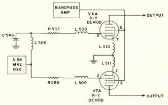
and amplitude differences of the two input signals into information that the color difference amplifier circuit can enlarge to magnitudes necessary for driving the CRT grids.
