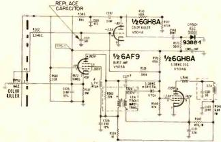
stitute this capacitor to determine if it has failed. Measuring it with an ohumeter may not reveal a defective capacitor. Replace with a  $.1\mu f$  of higher working voltage such as 64C53-98 ( $.1\mu f$ , 200v) which is now used in production.
