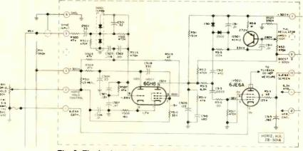
Fig. 6--The horizontal sync signal is fed to a conventional phase detector and is used to control the frequency of the horizontal multivibrator tube.
