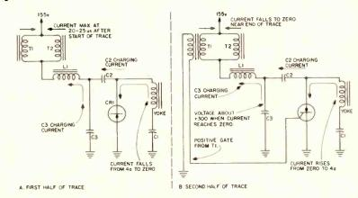
Fig. 5--Circuit action during trace interval.
