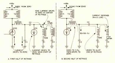
Fig. 3--Circuit action during retrace. First half of retrace is shown in Fig. 3A.
