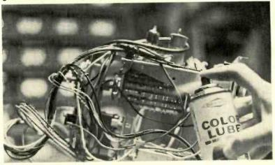
ed value or a capacitor going to ground is leaky or shorted. If the voltage change is intermittent, you can usually isolate the defective part by spraying components with freezing solution.
