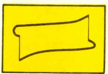
Fig. 8--Pattern showing phase shift and poor low frequency response.
