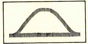
Fig. 2--Horizontal interference in the response curve caused by output tube radiation.
