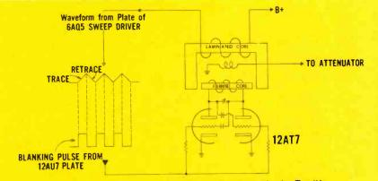
Fig. 3--Schematic of the sweep oscillator employed in the Zenith.
