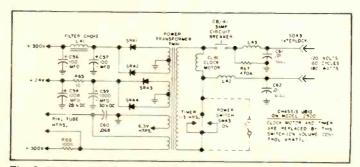
Fig. 8--As shown in the schematic, the 300v supply feeds only the deflection circuits. Video output circuits are powered from the 24v supply.
