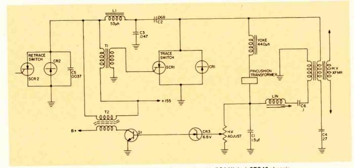
Fig. 1--Simplified schematic of the horizontal deflection system employed in RCA Victor'sCTC40 chassis.
