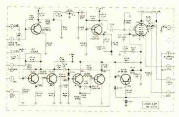
Fig. 3--Transistors Q203 and Q204 are connected as a Darlington pair and comprise the first chroma and sync amplifiers.
