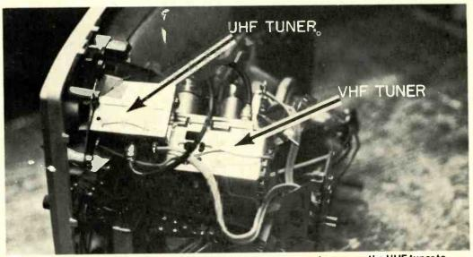
Fig. 3--In some sets, it may be necessary to remove the UHF tuner to get at the VHF.
