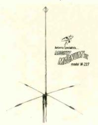
loading coils which electrically lengthen the radials to a full 1/4 wavelength thus producing a low radiation angle and a claimed 4db of omnidirectional gain. Other construction features include a waterproof coax connector jacket, chemically welded dual phasing coil jacket, and double-interlock dipole joints. The VSWR is rated at 1.05 to 1 at centerband and 1.4 to 1 at the band edges. List price is \$36.95. Antenna Specialists.
