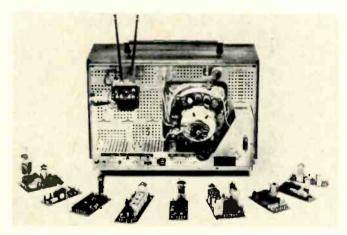
Over 90 percent of all circuit components are mounted on 10 plug-in units. Nine units plug into the chassis while the tenth mounts on the picture tube.
