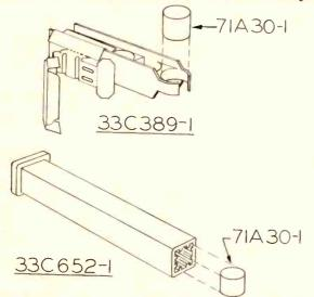
assembly of earlier color TV models. Order the type shown in the drawing. The magnet (71A30-1) is not included with either type. The mounting clip shown with 33C389-1 is included.
