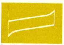
Fig. 6--The tilted or bowed pattern shows poor vertical low frequency response.
