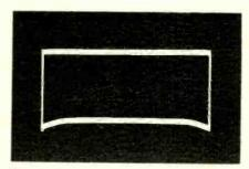
Fig. 5--A normal scope pattern with no phase shift and sufficient low frequency response.
