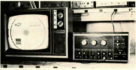
B&K Model 1077 television analyst, showing test pattern produced.
