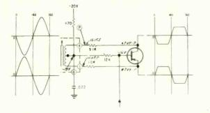
the upper 38kHz input wave supplies the positive bias from the emitter to the base on the first half-cycle. At the same time, the lower wave supplies the negative bias from the collector to the base. During the second half-cycle the reverse is true, but the action of the transistor is the same due to the bilateral effect.
