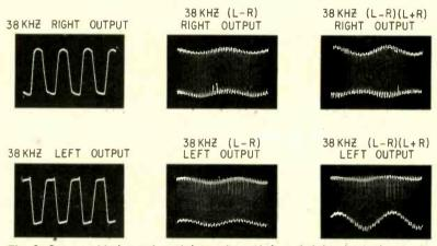
Fig. 2. Output of balanced modulator shows left and right channel outputs with 38kHz carrier.
