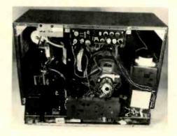
Rear view of chassis showing service controls.
