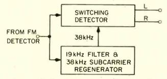
Fig. 4. Block diagram of a switching type FM receiver.
