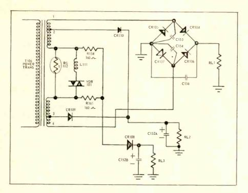
Fig. 5--Simplified schematic of the later balanced power supply.
