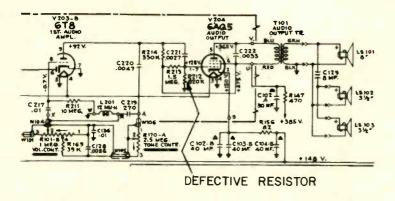
Fig. 5--Partial schematic of the audio section in the RCA Victor color chassis CTC5N showing the defective resistor causing audio distortion during color programs.
