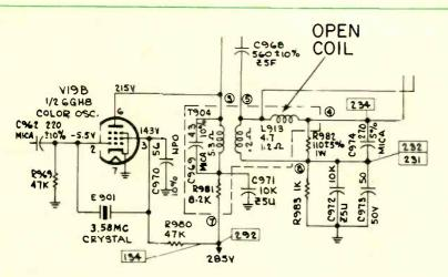
Fig. 1--Partial schematic of Motorola's TS908/Y color chassis showing open reference coil which caused no green color.
