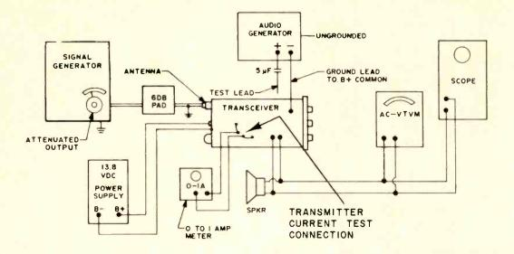
a signal generator ground lead must connect to an IF can shield, a part of the chassis mounting rail or to the metal ring of an earphone jack. It will pay you to observe the recommendations indicated in the transceiver's service instructions.
