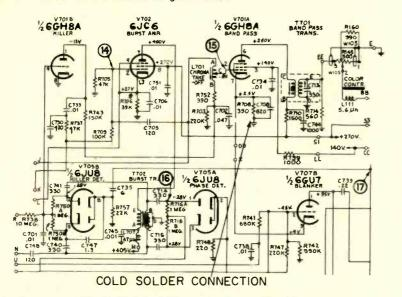
Fig. 2--The fading color and brightness level was caused by a poor ground connection in this RCA Victor CTC16 color chassis.
