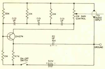
Schematic diagram of simple audio generator.
