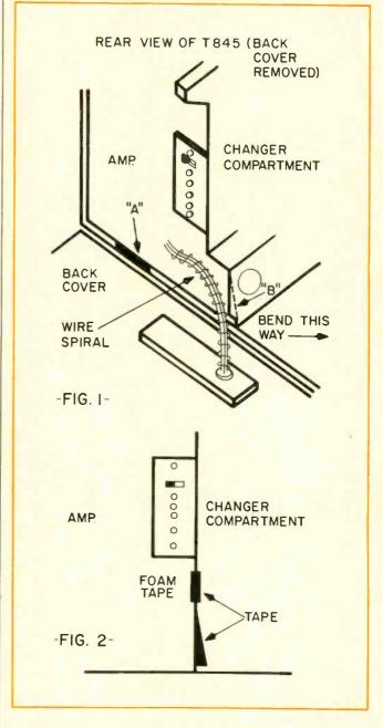
ac line cord strain relief and wire bundle. Insure sufficient spiral is used to cover cord. Note: Insure wire tie holding wire bundle is secure (See Fig. 1). Reinstall back cover observing ac lead dress to make sure that ac cord is dressed by taped area. Perform this normal safety check as follows:
