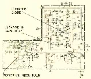
Fig. 3.—Partial schematic of the General Electric CB chassis showing the shorted diode which caused saturated green. The saturated red color was caused by a defective capacitor.
