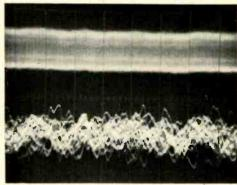
Fig. 14. The top trace shows the signal at the cathode of CR301 (Fig 10.). The bottom display is the audio output taken at point D in Fig. 9.
