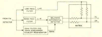
Fig. 3. Block diagram of a matrix type FM receiver.
