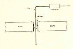
Fig. 1--The "Griplet," similar to an eyelet, has a grip inside holding components during the solder operation at the factory.
