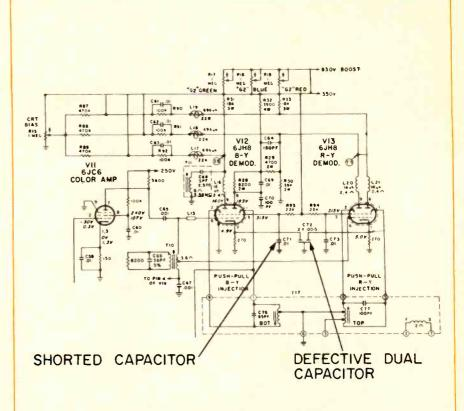
Fig. 4--The color section of a Zenith 24NC31Z chassis showing the defective dual capacitor causing weak red color reproduction.
