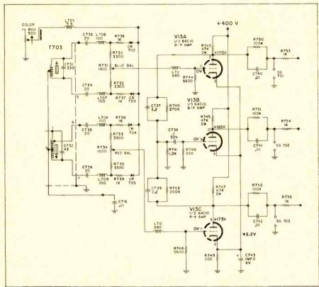
Fig. 3--Low pass filters are added in the grid circuits of the R-Y and B-Y color difference amplifiers.
