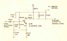
The inductance of the crystal itself with CD41, CD45 and CD46 forms an oscillator tank circuit which resonates at 3.58MHz. Working together, these components comprise a step-up effect between emitter and base. Since the base-emitter circuit of Q18 behaves as an oscillator, the emitter-collector circuit will amplify the 3.58MHz base signal.
