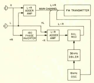
Fig. 1. Block diagram of an FM stereo multiplex transmitting system.
