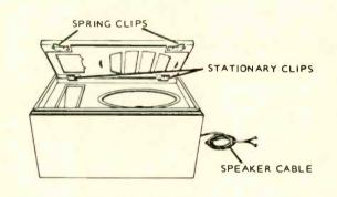
A dull-edged knife blade can also be used, but use care to avoid scratching the cabinet. The speakers are mounted from the front of the baffle board and sealed with caulking compound. The crossover network is mounted inside the cabinet. Therefore, the bass speaker must be removed to gain access to the network.
