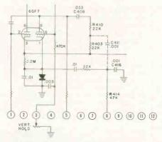
Vertical oscillator drift as the receiver warms up or vertical lock-in at the end of the vertical hold control range can be caused by a defective 12M resistor (R404) in the vertical hold circuit.
