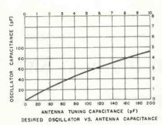
Fig. 11 — The desired combination of oscillator and antenna tuned circuit capacitances are shown for a transistor AM receiver. Courtesy of Motorola.
