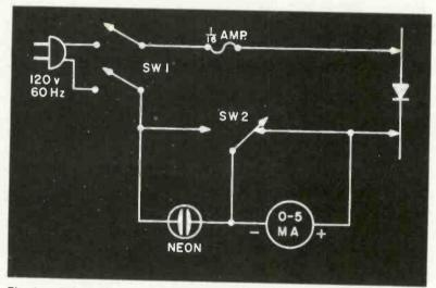
Fig. 4 — Schematic of test circuit used to check out focus-rectifier stacks.
