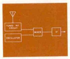
Fig. 5 — A superheterodyne circuit contains a variable-tuned radio-frequency (RF) circuit, a variable-tuned oscillator circuit and a mixer circuit, which produce an intermediate-frequency (IF) signal for additional amplification.
