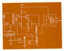
Fig. 12 — The varicap tuned, singletransistor circuit performs all the functions of a tuned oscillator circuit, tuned RF circuit and mixer circuit.
