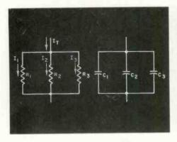
Fig. 7 - In both parallel resistor and parallel capacitor circuits, the total current passing through the circuit is equal to the sum of the currents passing through each component.
