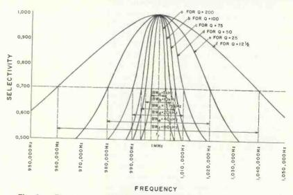
Fig. 4 — The greater a parallel-resonant circuit's quality factor (Q), the smaller the bandwidth (BW) of the resonant frequency.
