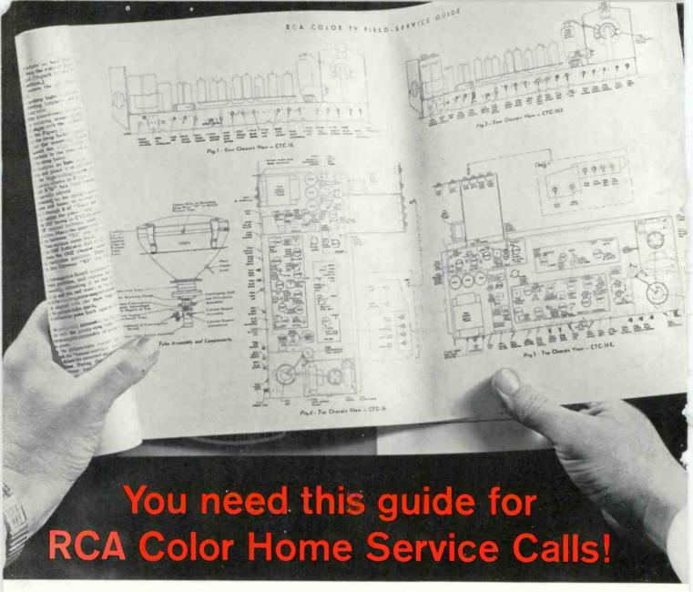
RCA'S NEW FIELD SERVICE GUIDE, ERT-200 helps you make all adjustments on all RCA color sets from 1955 to 1966 that can be performed in the home...including step-by-step procedure for replacing a color picture tube.
