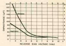
Fig. 15 — The capacitance in the antenna and oscillator circuits vary with the varicap reverse-bias voltage. Courtesy of Molorola.
