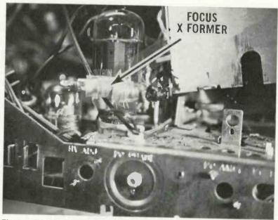
Fig. 3 — The focus transformer in this chassis went up in smoke.
