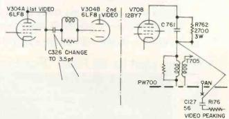
junction of T705 and C761 and R782. Change C326 PW300 board from a 5pf capacitor to a 3.5pf Stock No. 117531.
