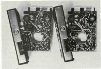
Fig. 13 — The underside of two AM transistor receiver circuit boards is shown. The left one is tuned with a mechanical-tuning capacitor and the one on the right is tuned with a varicap.
