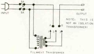
FILAMENT TRANSFORME 117V/12.6V,CT,5AMP 1. Purchase locally, a filament transformer with a 12.6v, center tapped, 5a secondary.
