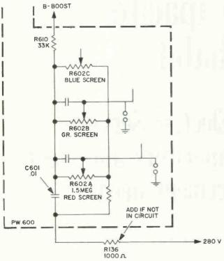
may also need replacement and R136, a 1K resistor (stock #502210) should be added in series with B+ as shown in schematic. Late production will include this resistor.
