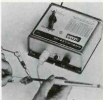
sule and a control unit that reduces the 120vac line voltage to the proper voltage for the desired temperature. The control unit includes a line-voltage meter, a power setting knob and a table that indicates the proper power setting for the line voltage and desired soldering iron temperature. Ungar.
