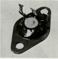
ratings reportedly are:  $V_{CEO} = 35v$ ,  $I_{C} = 3.0a$ ,  $T_{J} = -65^{\circ}F$  to  $+300^{\circ}F$ . Specifications indicate that the hFE is from 20 to 250 and 14.3w can be dissipated at 212°F. Bendix.
