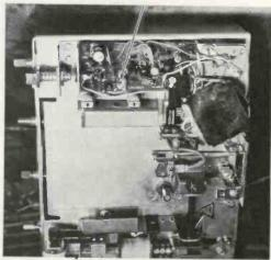
Fig. 7 — Speed can be adjusted on this player by adjusting the slotted speed control.
