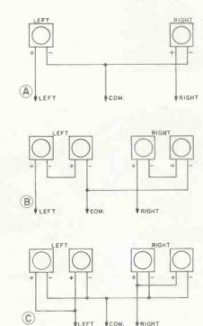
Fig. 5 (A) — Hookup for two 4 to 8ohm speakers. (B) — For four 4 ohm speakers. (C) — For four 8ohm speakers.
