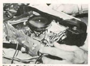
Fig. 9 — This Philco-Ford model tape player has a "shiny" belt and flywheel. Slow or erratic speeds can be eliminated by cleaning the glaze and oxide dust from belt, wheel and tape drive assembly.
