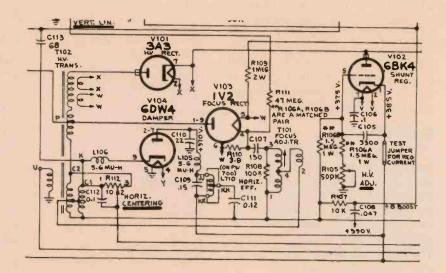
Fig. 2 — HV section of Zenith 20X1C36 color chassis showing selenium rectifier and adjustable pot used in focus voltage circuit.
