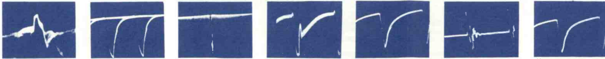
6 TP501 60V P-P (HORIZ.) SYNC SEPARATOR GRID 7 JUNCTION R516 & R545 70V P-P (HORIZ.) SYNC SEPARATOR PLATE 8 JUNCTION R516 & R545 80V P-P (VERT.) SYNC SEPARATOR PLATE 9 COMMON CATHODE 13V P-P (HORIZ.) HORIZ. PHASE DETECTOR 10 V503-9 (C515) 300V P-P (HORIZ.) HORIZ. OSCILLATOR GRID 11 TP503 300V P-P (HORIZ.) HORIZ. OSCILLATOR COIL 12 PW500W 300V P-P (HORIZ.) HORIZONTAL DRIVE
