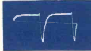
4 V201 PIN 1 SYNC PLATE HORIZONTAL RATE 55V P-P
