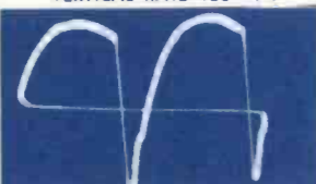
11 SR201 CATHODE JUNCTION HORIZONTAL PHASE DETECTOR HORIZONTAL RATE 13V P-P
