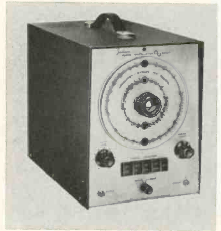
Jackson Model 605D audio sine/squarewave oscillator.
