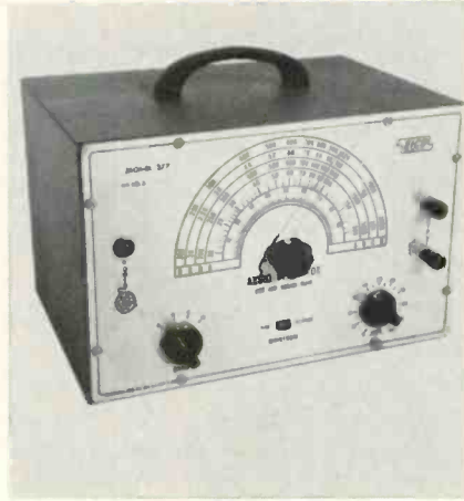
Eico Model 377 sine/squarewave generator.
