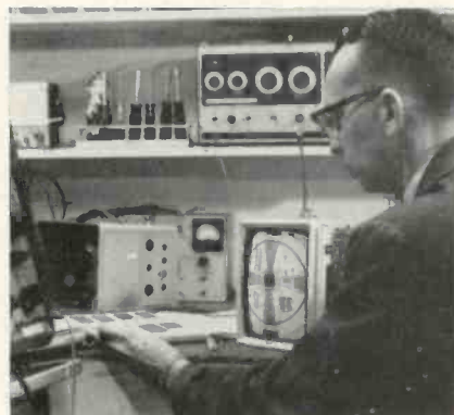
Fig. 8—Using the "analyst" to isolate trouble by signal injection.
