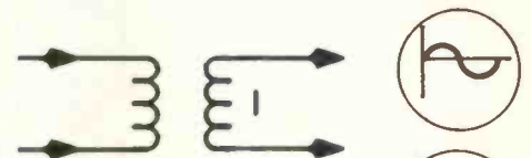
Fig. 5—The voltages present at the transformer's two secondary leads are 180deg out of phase.
