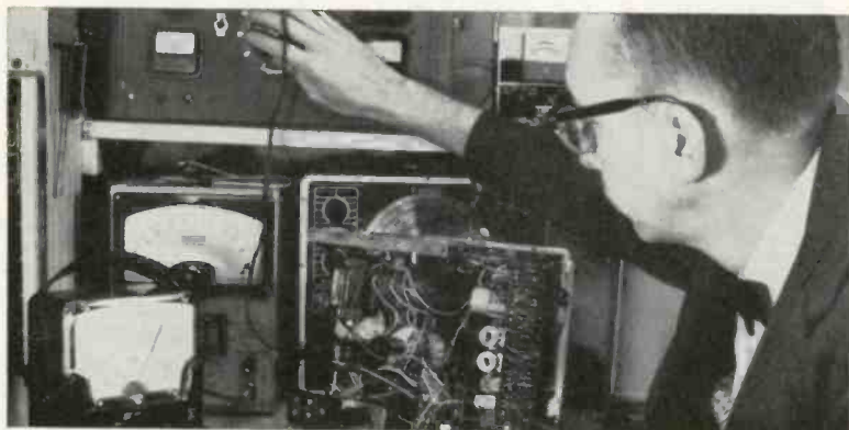
Fig. 2—The "old pro" uses a variable ac power supply to bring up the line voltage slowly when checking for shorts and overloads.
