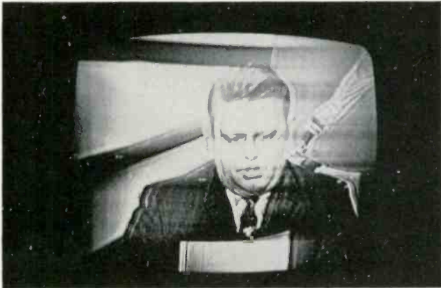
Fig. 10—Triple image caused by an open choke, L9, in a Zenith 23xC36 chassis.
