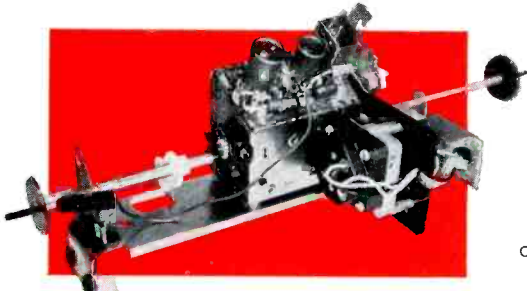
Fig. 2—The tuner assembly is easily detached by removing two mounting bolts.
