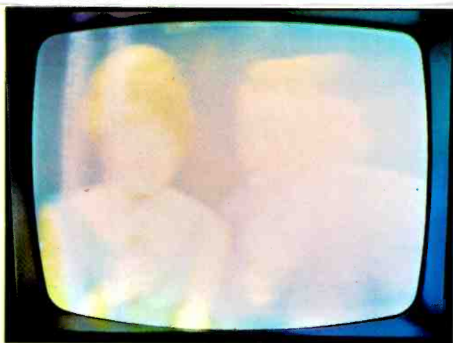
Fig. 4—Burned or carbonized HV isolation resistor can cause out-of-focus picture and lines on screen.
