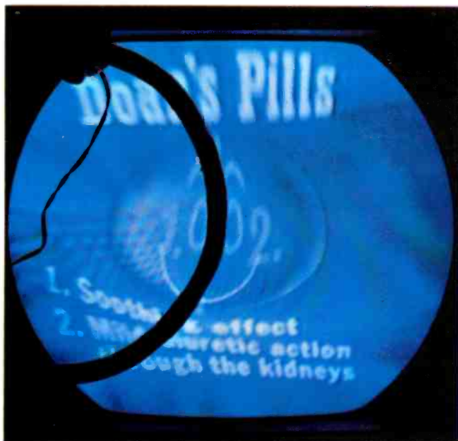
Fig. 6—Using service degaussing coil to isolate a defective ADG system.
