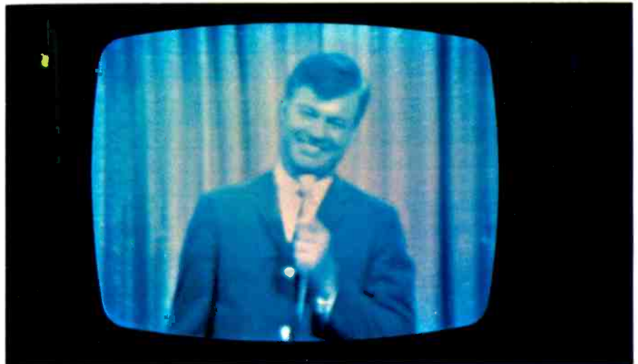
Fig. 1—Color phase problem. Note the faces are blue. Correct facial tint could not be obtained.
