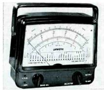
function indicator which visually indicates the exact range being used. The meter is  $6\frac{1}{2}$  in. wide with a two color, full range  $90^{\circ}$  arc. The VOM includes built-in protection against burnout and bent pointers. Dimensions,  $7\frac{1}{8} \times 6\frac{3}{8} \times 3\frac{1}{8}$  in. Meter movement sensitivity,  $9\mu$ a for full scale deflection. Price \$44.95. Lafayette.
