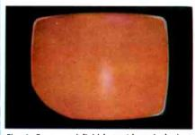
Fig. 4-Proper red field but with neck shadow.
