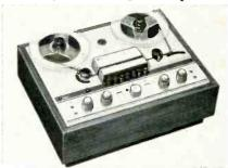
The die-cast mainplate features 3 motors and the brakes, tape gate and pinch roller are solenoid-operated. There are 3 tape heads for erase, record and playback plus a 21 transistor, 4 diode amplifier. Price \$399.50. Heath.
