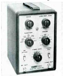
can be connected directly to the set's antenna without requiring gun killers. Size  $8\frac{1}{2}$  x5\frac{3}{4} x6\frac{3}{6} in. Price \$169. EICO.
