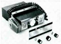
knobs and two shaft nuts from its front panel controls. The panel can then be lifted away, exposing the bank of crystal sockets and channel indicator dial. Receiver image rejection is rated at 50db, and sensitivity at 0.4 mv for a 10db s/n ratio. By turning the transceiver's squelch control completely counter-clockwise, the audio output circuitry is changed into a public address amplifier. Dimensions,  $2\frac{1}{2} \times 6\frac{1}{2} \times 9$  in. Price \$179.95. Amphenol.
