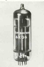
design characteristics developed to eliminate Barkhausen oscillations. As a result, the manufacturer claims snivetsuppression circuits can be eliminated, resulting in lower circuit costs. Maximum peak plate, 7000v. Maximum plate dissipation, 34w. Peak anode current, 1.4a. Ampex.
