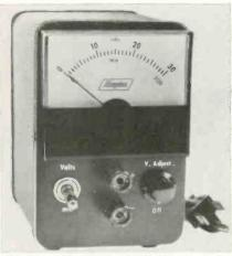
300ma over a range of 1.25 to 30vde with a load regulation of  $\pm 0.5\%$  or 50mv, whichever is greater; has a 10mv line regulation over a range of 105 to 125v and a full load ripple of lmv RMS. It stands 5% in. high and weighs 3 lb. Acopian Corp.
