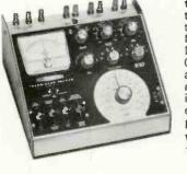
Complete Service / Laboratory Transistor Analyzer ... the Heathkit IM-30 provides thorough DC analysis of PNP & NPN transistors. Test for shorts, DC gain (Beta 0-300) (Alpha 0-0.9967), Leakage (Icbo, Iceo), and diode forward & reverse current. Requires 7 "D" cells for internal power — provisions for external power.
