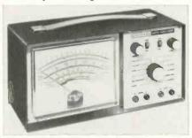
all automotive and boat engines. The comprehensive manual lists the idle speeds and the dwell angles for both manual and automatic transmissions. The analyzer is useful for all 6 or 12v; 4, 6, or 8-cylinder engines with negative or positive ground. Eico.
