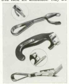
used for slitting most types of cable jackets, especially the outdoor heavyduty types; stripping the jacket from all sizes of inside types of plastic and fabric covered cable; and "ring" cutting the sheathing of inside types plastic, fabric or rubber covered cable. The cut through the sheathing is limited to 1/32 in. for protecting the wires. P. K. Neuses, Inc.
