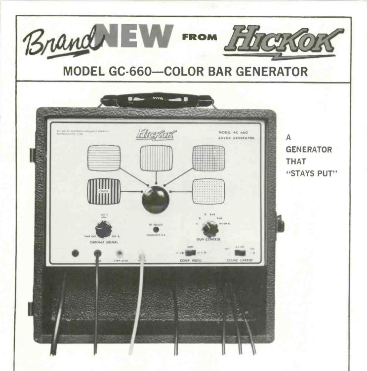
• A proven, field-tested design • "Stays put"—designed for Alaskan cold and Florida heat and humidity\* • 0.1  $\mu$ sec dots—plus a crosshatch pattern that doesn't "flicker" • Standard gated color bars at zero reference level—for correct color phasing adjustments.
