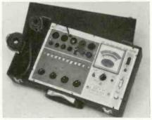
for proportionate screen brightness by qualitative measurement of the electron beam. The central area of the picture tube cathode is checked in addition to the controlling action of the first grid. The instrument weighs 8lb and measures 16 x 9 x 4<sup>3</sup>/<sub>4</sub> in. Net price \$92.95. Precise. Insist on Genuine RCA Replacement Parts...
