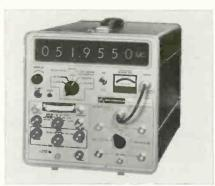
plays a seven digit in-line read-out with four automatic decimal points and indicates whether the read-out is in Hz, kHz or MHz. Motorola.
