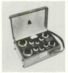
accuracy of 3% from 535 kHz to 1605kHz. The signal generator is said to have a calibrated output from 10mv to 1v with an accuracy of  $\pm 1\%$ , and frequency range of from 535kHz to 1605kHz with a readout accuracy of  $\pm 3\%$ . The monitor receiver is designed for sensitivity of better than 5mv, weight, 12 lb. Wilkinson.
