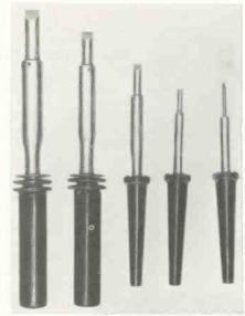
style irons. In addition, two larger general types of 120w and 175w are offered. The entire line features stainless steel barrels, heat and impact resistant handles and light weights. Weller.
