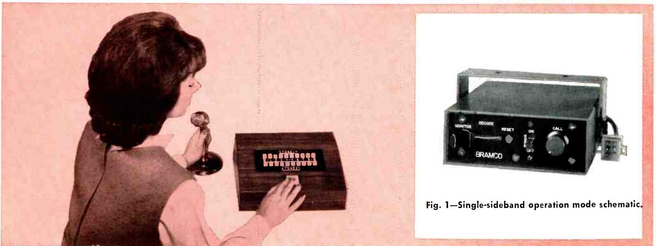
Fig. 4: 90-code selective calling encoder console generates two-tone sequential signals. Decoder alerts selected mobile receivers. Courtesy Bramco.
