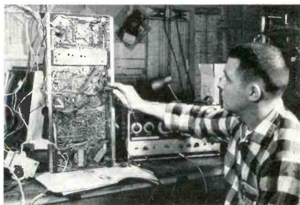
Technician Messerly checks sync circuit in a color set with 'analyst.'
