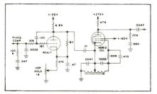
Fig. 1—Philco 16QT85 horizontal oscillator and reactance circuit
