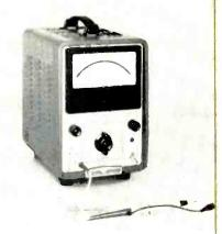
Fig. 3—Pico-ammeter and micro-voltmeter has a full-scale dc current range of 10pa. The current of 10pa is measured as a voltage drop of 10μν across an internal 1M resistor. Hewlett-Packard model 425A.
