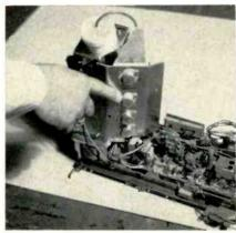
Power transistors are often mounted together on a common heat sink. Some are insulated from the sink.
