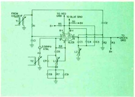
Fig. 1 — Oscillator-demodulator circuit employing 6LE8
