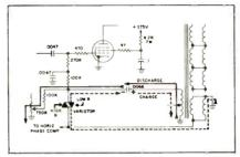
Fig. 2—Horizontal output circuit bias
