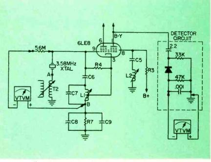
Fig. 2-Detector circuit used for aligning 3.58MHz trap in demodulator outputs
