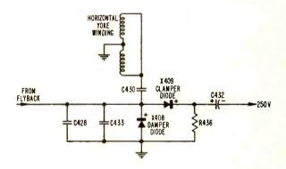
The entire pulse lasts for about  $22\mu$ sec of the total horizontal scan time of  $63\mu$ sec. This time, then, represents the "on" time of the oscillator.
