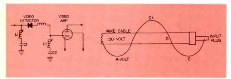
Fig. 2—Series-tuned traps inserted in both video detector and video amplifier circuits Both are tuned to 222MHz.
