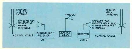
Fig. 2—Combination simplex and duplex marine radio system.
