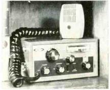
verts the 650 to a public address system when used with an external speaker. With 12vdc and 115vac power supplies it measures 33/4 x 63/4 x 91/2 in. Amphenol.
