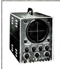
sensitivity specified as 0.053v RMS/in. on the wideband position and 0.018v RMS/in. when the switch is in the more sensitive narrow band position. Risetime is stated to be  $0.1\mu$ sec when the passband switch is in the 4.5MHz position and  $0.5\mu$ sec when the passband switch is in the 1.5MHz position.
