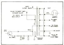
Fig. 3—Horizontal output transformer circuit details
