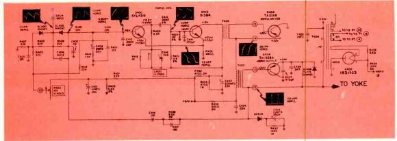
Some horizontal systems look foreign in transistor sets. The output transistor generally feeds the voke directly.
