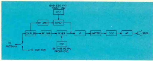
Fig. 1-Some VHF receivers have two front ends.
