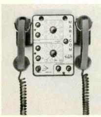
Control unit for multi-channel VHF/FM marine radiotelephone by Comco.
