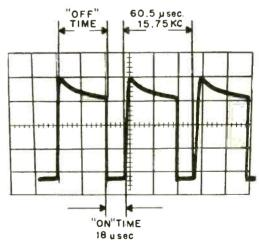
Figure 6-Waveform at TP4
