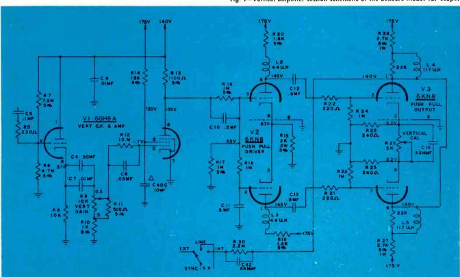
Fig. 1—Vertical amplifier section schematic of the Sencore Model 127 scope.
