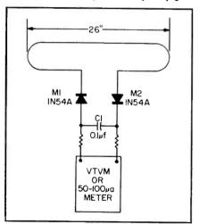
Fig. 5—Simple strength meter for measuring intensity of radar signal.
