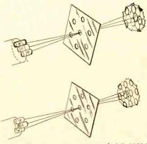
(Top) In-line gun arrangement of G-E 11SP4 color CRT. (Bottom) Gun arrangement in conventional color CRT
