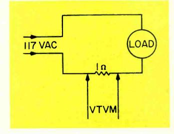
Fig. 2—Method of measuring current in an ac circuit.
