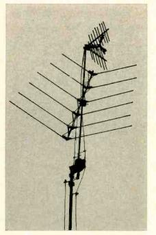
Rotor-operated antenna gives excellent results in one area-picking up all UHF channels in the area (channels 21, 25 and 49).
