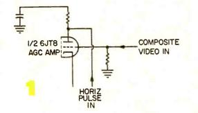
Fig. 1-Simplified typical AGC circuit.
