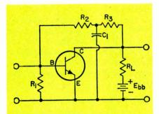
Fig. 2(A)—Bias network in common-emitter circuit uses emitter stabilizing resistor. (B)—Common-emitter circuit using splitvoltage-divider bias network.
