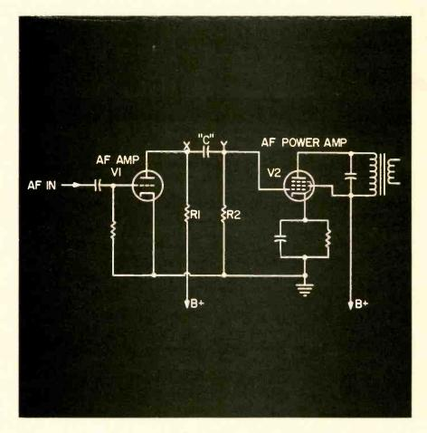
Fig. 3-Method of measuring dc leakage in audio coupling capacitor.
