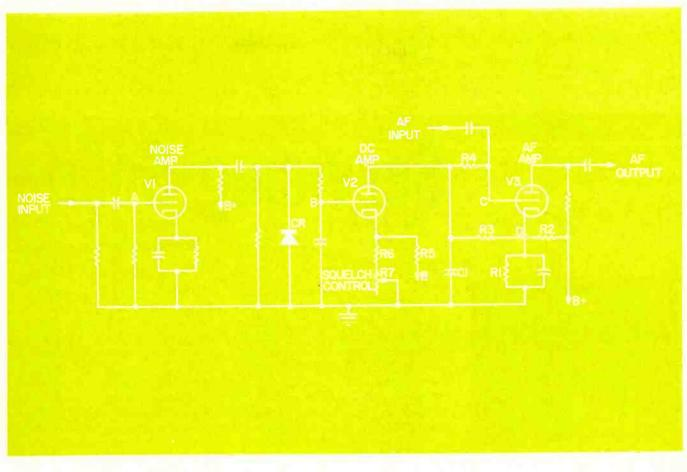
Fig. 4-Typical squelch circuit in two-way communications receiver.
