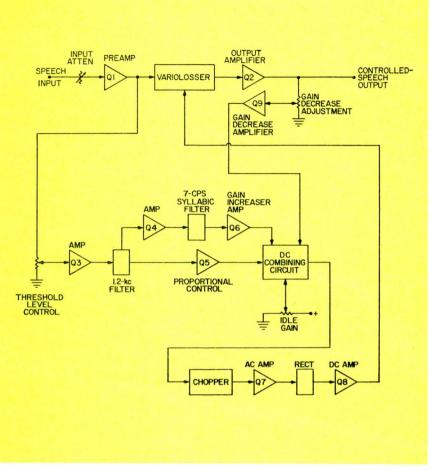
Fig. 1-Block diagram of AGAMP.
