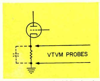
Fig. 1—Measure dc voltage across the cathode bias resistor and use ohm's E/R formula to determine approximate current.
