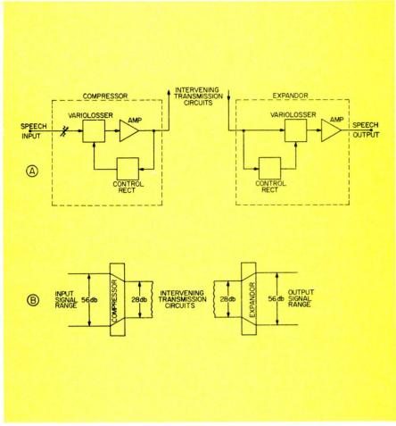
Fig. 2—The Compandor. (A)—Compressor and expandor sections. (B)—How signals are compressed and expanded.
