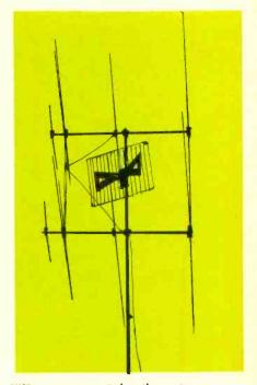
UHF antennas mounted on the mast in this position can and usually will give erratic reception.
