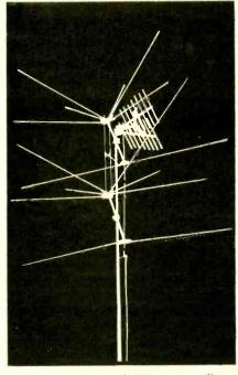
Fig. 2—A well-mounted UHF corner reflector gave poor reception because of losses in ordinary twin-lead.
