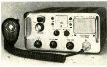
cluding compactrons and nuvistors. It has a built-in power supply for 12 or 115v operation. The unit is an upper sideband, lower sideband or double sideband transceiver. General.
