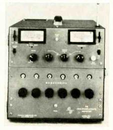
nounced. The CE1 has direct reading offered on all bands: 20-80Mc, 120-180Mc, 420-480Mc, and 920-980Mc. Three directly calibrated frequency and three directly calibrated deviation ranges are included. The self-contained, portable instrument measures 10 3/4 x 10 5/16 x 16-1/2 in. Cushman Electronics.
