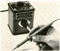
ing iron which utilizes regular tips is announced. The power-control unit's range of 350-750° tip temperatures is set by a direct-reading dial. American Beauty.
