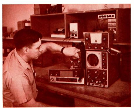
Typical bench set up using the audio generator, signal tracer and modified scope. Photo and diagrams Courtesy Heath Co.
