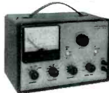
New Model 378 Audio Generator. Near-distortionless sine wave generator (< 0.1% 20-20,000c) providing fast, convenient, switchable selection of frequencies from 1c to 1,000c (1c steps 10c-100c, 10c steps 100c-1kc, 100c steps 1kc-10kc, 1kc steps 10kc-100kc). 8-pos. 10db/step output attenuator & fine attenuator. Output meter (4 1/2" 200ua) with 8 voltage ranges & db scale. $49.95 kit, $69.95 wired.
