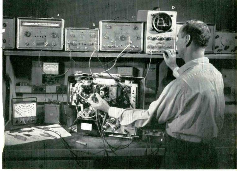
Checking overall frequency response (RF and IF) in a portable B&W TV receiver using the test instruments described below. Pattern on oscilloscope screen is an overall response curve with dual markers: one at picture-carrier frequency and one at sound-carrier frequency.
