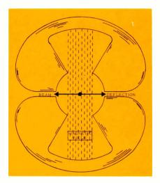
Fig. 2—Basic reflection principle for horizontal winding as shown in Fig. 1A. The complex magnetic lines-of-force pattern has been greatly simplified to show basic winding deflection.
