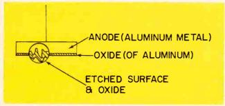
Fig. 4—When oxides are formed on most any material they will act as an insulator.
