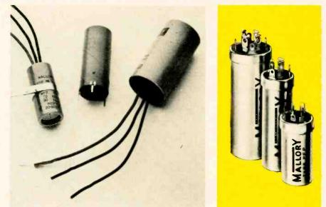
Fig. 3—Early version of wet electrolytic had folded 'accordion' aluminum anode.
