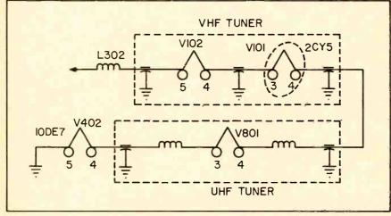
Intermittent cathode to heater short in tuner tube caused lack of vertical sweep in Admiral 15UA2 chassis.
