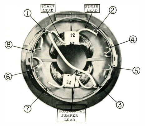
Fig. 3—Rear view of a 110 deg yoke with cover removed. Terminals are indicated by circled numbers. Note leads to terminals 6, 8, 5 and 4—vertical windings—not visible in photo. The vertical jumper lead has been omitted for clarity too.
