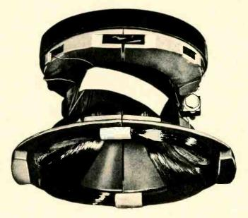
Fig. 5—Yoke with toroidal wound vertical windings, common in some late TV receivers.
