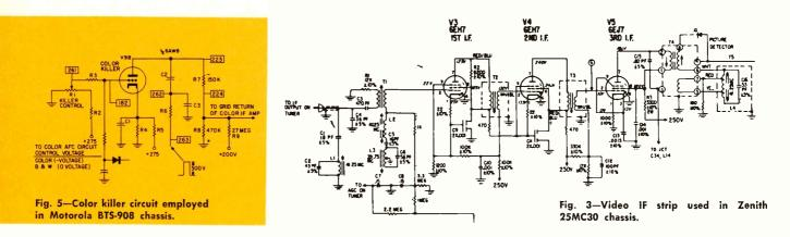
quencies. The wideband response is achieved by stagger tuning and the addition of properly designed filters and traps. Early color TV sets contained up to five video IF stages but higher gain frame grid tubes made it possible to employ only three and sometimes as few as two IF stages in newer designs.
