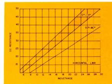
Fig. 4—Relationship of L and R values in typical series connected horizontal yoke windings. Assuming a 110 deg yoke measures 35 ohms across the horizontal winding, then the chart can be used to determine that the inductance is 17 to 21 mh for a typical yoke of this type. A standard replacement with a 35 ohm, 18 mh winding should be suitable. A chart like this is not necessary for vertical windings since the resistance (in ohms) very nearly equals the inductance (in mh) for all types.
