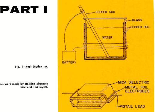
Fig. 2-Original capacitors were made by stacking alternate
