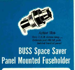
• Fuseholder takes  $\frac{1}{4} \times 1\frac{1}{4}$  inch fuses. Converts to  $\frac{9}{22} \times 1\frac{1}{4}$  inch fuses simply by changing screw type knob. Holder is rated at 30 ampere for any voltage up to 250.
