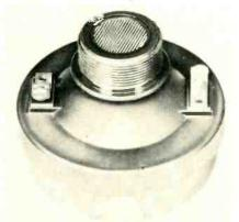
Power, 20 w. Impedance  $16\Omega$ . Frequency response, 120-7,000 cps. Sound level, 125 db measured 4' on axis at rated power with 6' air column. Driver threads, 13% in.-18 standard. Atlas Sound.
