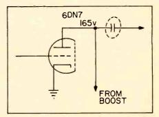
Shorted capacitor in vertical circuit disables HV of G-E M-6 chassis.
