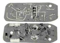
UNRETOUCHED PHOTOS OF PRINTED CIRCUIT AND POTTED COMPONENT SIDES OF TELE-AMP AMPLIFIER BOARD AFTER 204-HOUR WEATHER-TORTURE TESTS
