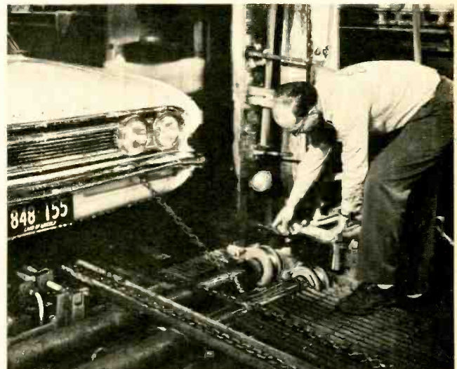
Track can be restarted only by radio transmitter, preventing accidents while repairs are being made.
