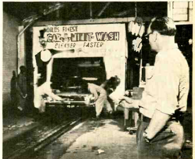
Car wash track is stopped by remote control from hand-held radio transmitter.
