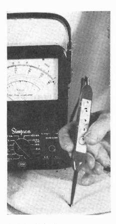
Fig. 5—Speedprobe allows selection of voltage ranges on the probe. A wide range of special probes are available.
