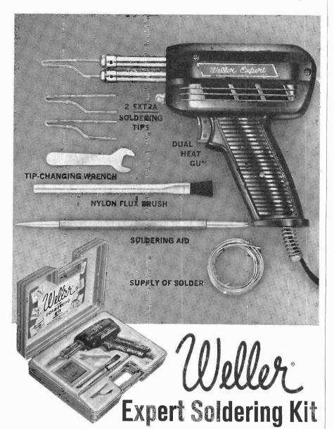
All your soldering needs in a break-proof plastic utility case. Gun features dual heat. 2 trigger positions permit instant switching to low 100-watt or high 140-watt heat. Low heat prevents damage to heat sensitive components. By using high heat only when necessary, you prolong tip life and save current.
