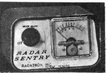
transistors and 2 diodes mounted on print circuitry and housed in a durable, interference-free magnesium case. Completely portable, it operates on two 1,000 hour, self-testing mercury batteries. The instrument is capable of receiving cw signals and all other types of modulation over a frequency range from 1000 Mc, in the "L" band, up through 11,000 Mc, in the "X" band. It is sensitive to signal levels as low as -65 dbm. Detection of radiation is indicated by an audible
