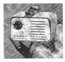
Ingenious, miniature electronic detector gives audible warning of approach to radar-timed speed zones and dangerous areas protected by radaroperated signal lights.
