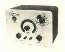
resistance ranges from 1 ohm to 150 megohms; fully variable d-c voltage up to 450v; 1% precision resistors; 5% capacitors and 6E5 null indicator tube. Kit, \$19.75. Assembled, \$28.75. National Radio Institute, 3939 Wisconsin Ave., Washington 16, D. C. For more data, circle 11-66-3 on coupon, p. 50
