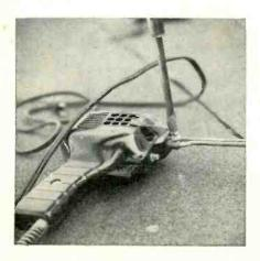
Fig. 1-Keeping screws (or lock nuts) tight will solve most slow and poor-heating tip problems on solder guns.
