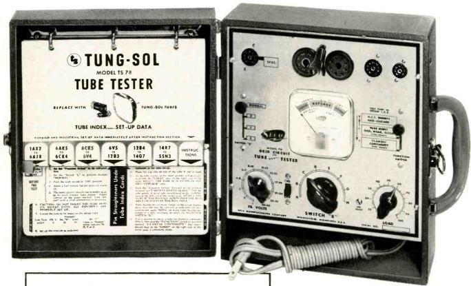
The Model TS-78 Tube Tester is a precision instrument, exceptionally fast and easy to use. Five sockets accommodate all tubes.
