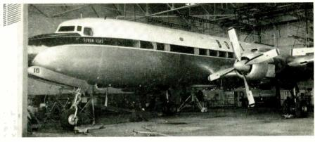
Fig. 4—Heavy aircraft is weighed by mounting strain gages on ram jacks under each wheel. Aircraft's center-of-gravity can also be determined in a similar manner.
