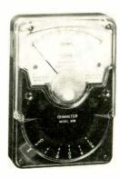
0-2 megohms; 0-20 megohms (20 ohm center scale on 0-2000 range). Tester,  $2\frac{3}{4}$ " x  $4\frac{1}{4}$ " x  $1\frac{1}{16}$ " fits into the palm of the hand and has back mounted elastic strap and control knob. Triplett Electrical Instrument Co., Bluffton. Ohio.
