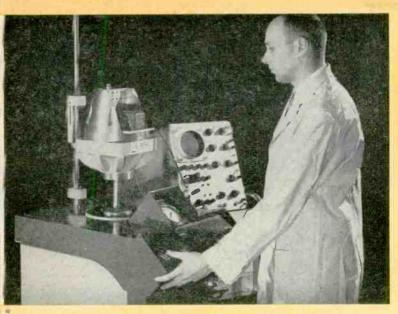
Avco shock test machine for electronic components tests a relay with a 30 g, 31 millisecond half-sine shock. It can test up to 3000 g. There is no superstructure, and the machine relies on air pressure to propel it down during test.
