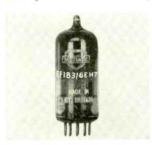
low microphonics; internally shielded; and proven reliability and trouble free performance. Characteristics EF183/6EH7, a variable-mu r-f pentode: transconductance, 13,000 micromhos; plate voltage, 200v; plate current, 12 ma; heater voltage, 6.3v; and current .3 amp. International Electronics Corp., 81 Spring St., New York 12, N. Y.
