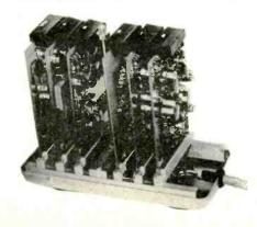
Fig. 6—Budelman mone-bloc used in 2000 mc microwave transmitter, provides a stable, broadband, and high Q output circuit.
