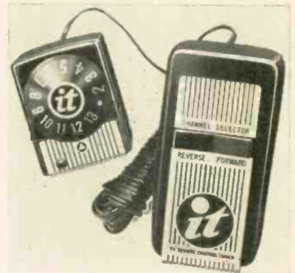
"It" drive motor (l) mounts on tuner shaft. Batteries are in remote control box (r).
