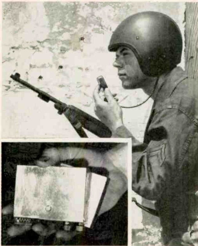
Cpl. Harry Mikus reports back to his squad through tiny combat radio built into his helmet. Mike slips under helmet when not in use. Rugged FM radio (inset) developed by Signal Corps weighs 1 lb., uses transistors, has 1 mi. range with auxiliary antenna atop helmet. Without this antenna, it is preset for short range to prevent enemy interception. U. S. Army photo.
