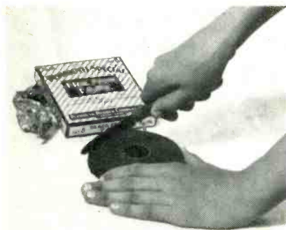
Prevent tape fraying by scoring the roll.
