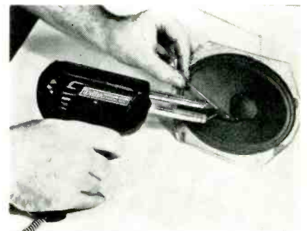
Fig. 5—Resoldering the severed connection of a voice-coil lead to paper speaker cone.
