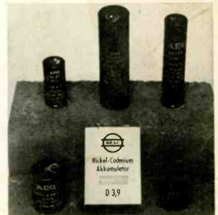
Fig. 3—Typical "canned" selenium bridge rectifier units. The large center object is the "accumulator" or battery for the portables.
