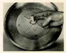
Fig. 2—Lubrication of the turntable shaft,
