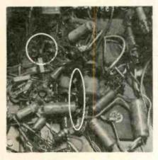
Fig. 2—Inadequate repair of fire damage: Charred tube socket not replaced (resistance reading possible from any pin to ground); damaged terminal strip not replaced; ends of burned-out resistors left harging in set; charred resistors, capacitors not replaced.
