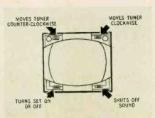
remote control system which permits the customer to change channels, turn the set on and off, or turn down the volume, just by hitting the appropriate photo-electric cell with the beam from the flash-gun provided.
