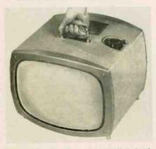
Newest in the line of Setchell-Carlson's "Unltized" TV receivers, this portable version has all-aluminum construction of both chassis and cabinet. Weighs less than 40 lbs., yet boasts power transformer, keyed AGC, cascode tuner, 6-in. speaker and 90° aluminized 17-in. crt
