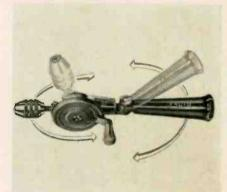
chuck and handle are adjustable to various angles, so that the drill will reach around obstructions, work close to floors and walls, and operate in close quarters: The 0 to  $\frac{1}{2}$  in. capacity chuck swings in a 270° arc, and has a spring lock that enables the user to change angles with a flip of the thumb. The handle turns in a 180° arc at right angles to the chuck movement path. Plomb Tool Company, Los Angeles, Calif.—TECHNICIAN (Ask for No. 7-4)
