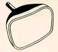
than that used in the face plate. Otherwise, when the neck is heated to seal in the mount, impurities may be given off which could contaminate the tube. Thus, renecking is necessary right at the start, to provide a bulb of suitable characteristics.
