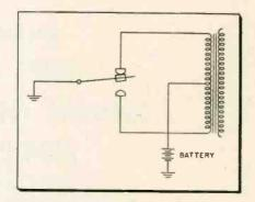
Fig. 2-Switch action makes ac of battery dc.
