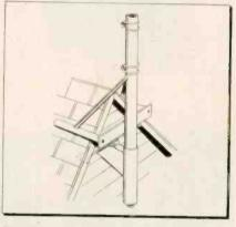
Simply loosen bottom bolt, slip mount into place, and then tighten bolt. Accommodates tubing up to 1½ in. in diameter. Rohn Mfg. Co., 116 Limestone, Bellevue, Peoria, Ill.—TECHNICIAN (Ask for No. 7-11)
