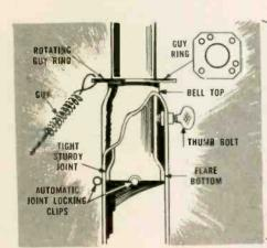
Comes complete with optional base—rotating guy rings for 3 or 4 guy points. MB-1 Standard Base for mounting on flat, vertical, sloping, or peak roofs.
