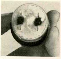
Tube appears new but internal "burn" marks are tip-off that it has seen heavy usage
