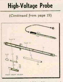
The h-v probe (upper right) and its component parts, showing various arrangements possible.
