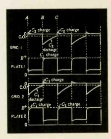
Fig. 2—Grid and plate waveforms for both triodes of a normally operating multivibrator.
