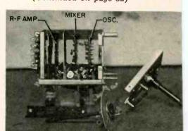
Fig. 5—RCA type KRK-8, shown disassembled, is an "incremental inductance" tuner.
