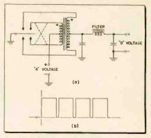
Fig. 5A—Circuit of synchronous or self-rectifying vibrator. B—Pulsed output waveform.
