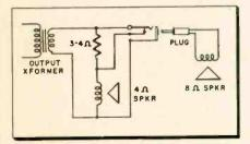
Fig. 1—Extra 8-ohm speaker at viewer's chair plugs into matched 4-ohm audio output.
