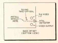
Anti-buzz shielding for sound take-off coil.
