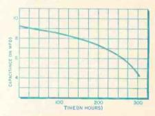
Fig. 2—High temperatures reduce capacitance, also increase condenser's series resistance, thus reducing bypassing efficiency. Motorboating or low-freq. oscillation may result.
