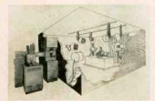
New setup uses beam from crt to scan scene, with reflected light being picked up by multiplier phototubes, eliminating iconoscope.
