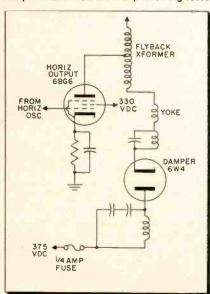
horizontal and high-voltage sections were replaced, a new fuse was installed and the cap of the 1B3 high-voltage rectifier was lifted. The set was turned on to check the cap of the 6BG6 for an arc, and the fuse again blew. The plate cap of the 6BG6 and the fuse were both removed to take B-plus off the plate and screen grid respectively. An oscilloscope check showed the horizontal pulse was present at the control grid and appeared to be normal.
