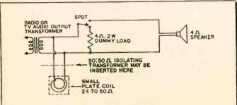
Fig. 3—Inductive wiring for entire room allows free movement of hearing aid wearer about room while he listens to TV sound output.
