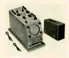
coupled amplifiers in both vertical and horizontal circuits. Fully compensated horizontal and vertical attenuators. Vertical bandpass—dc to 4 mc; horizon tal-dc to 500 kc. Input impedance to vertical amplifiers is 2.2 megohms-25 μμf. Hickok Electrical Instr. Co., 10523 Dupont Ave., Cleveland.—TECHNI-CIAN (Ask for No. 6-42)
