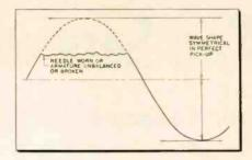
Fig. 4-Distortion due to defective pickup.
