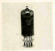
a video amplifier. The triode section has a mu of 18 and is suitable for applications where a low-mu triode is desirable, such as sync amplifiers, etc. Sylvania Electric Products, Inc., 1740 Broadway, New York 19, N. Y.—TECH-NICIAN (Ask for No. 6-75)
