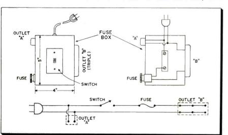
This fuse box on the service bench can save a lot of time when shorts occur in faulty chassis.
