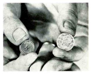
Thumbnail size mercury battery has smaller diameter than a dime.
