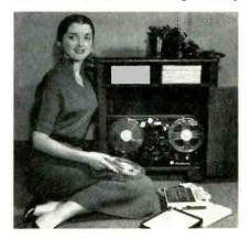
music systems. The unit (SRT-1) is electrically matched for use with all combinations of RCA intermatched hi-fi electronic components; utilizes all types of standard magnetic tapes, in 5-in. and 7-in. reels; and is designed for halftrack recording. It can be installed in either vertical or horizontal position. \$325. Engrg. Prods. Div., RCA, C. inden, N. J.—TECHNICIAN (Ask for No. 4-12)
