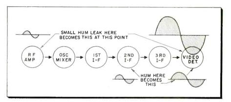
Fig. 4—Hum originating at the front of the receiver is amplified by succeeding i-f stages.
