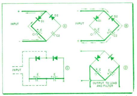
Fig. 2-How a voltage can be stepped up with the bridge-type doubler power supply.
