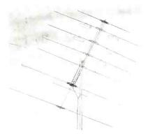
low band channels. All elements are in the same plane, providing extremely rigid construction; no boom braces are required on the  $1\frac{1}{2}$ -in. crossarm. The antenna was designed for fringe area reception. Elements are completely factory assembled by means of a springloaded quick rig design. Technical Appliance Corp., Sherburn, N. Y.--TECH-NICIAN (Ask for No. 4-20)
