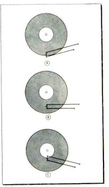
Fig. 2—How arm tracks across surface of disc.
