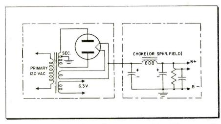
Fig. 1-Full wave power supply. Sources of 60 cps hum are at left; of 120 cps hum at right.
