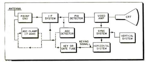
put to the picture detector reasonably constant, then too much variation may be present in the sync take-off, with consequent sync trouble due to a form of overloading. Some manufacturers employ an adjustable trimmer condenser to cut down the sync input. This is called the 'sync locking range' adjustment, and it helps compensate for agc deficiency.
