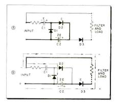
Fig. 3—Operation of the half-wave tripler.
