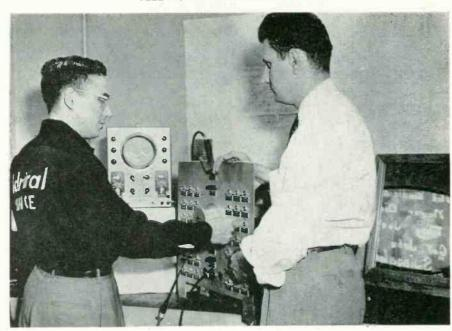
'Dynamic Illustrator' TV receiver, shown at Admiral's national service dept., inserts any one of 21 stock TV troubles at the flick of a switch. Additional switches permit observing the troubles on a scope. Rig was put together by Admiral service engineers for their training schools.
