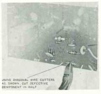
Fig. 2—For extra length you can use the section normally buried within the component.
