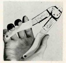
bolt, and screw sizes. The Champ is made of heat-treated steel and equipped with insulated handles. Wire and screw sizes, as well as the stud gauge and a stripping gauge, are etched on permanently. Aircraft-Marine Products, Inc., 2100 Paxton St., Harrisburg, Pa.—TECHNICIAN
