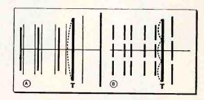
Fig. 2A—Yagi using a tripole, T, as the driven element. Low-band parasitic system is shown by heavy lines, high-band system in light outline. B—High-band operation. Low-band elements are not shown.
