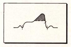
Fig. 2—Peak in response. Signals in the frequency range represented by the shaded area tend to cause spurious oscillation.
