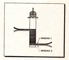
Fig. 3—Bifilar type of i-f transformer. Either winding may be used as primary or secondary. Powdered-iron slug tunes coils.
