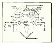
Fig. 4—Bridge circuit of Fig. 3 shown in more detail.  $R_{\rm p1}$  and  $R_{\rm p5}$  are tube plate resistances.
