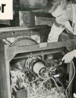
♥ After four months of servicing these sets, shop techs have a word of cheer—the standard troubles, sync and supply voltages, are still most common. Color circuits give little trouble ♥ Aligning the color receiver for the full 4 MC bandwidth requires careful adjustments-and top-notch equipment. Run-down sweep generators and marker generators will need re-calibration
