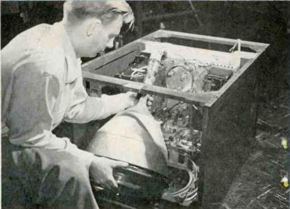
A Tri-color tube is easily installed by laying cabinet face down on floor, with top removed.  $\mu$ -metal shield shown around CRT prevents stray magnetic fields from affecting convergence, smearing colors
