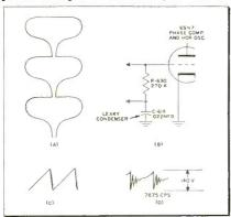
B). The waveform at the grid was a normal-appearing sawtooth (see illustration C) with slight jaggedness on the retrace portion of the waveshape. The defect in the waveform eluded me until I compared it with the correct grid waveform in the service data and schematic for the set (illustration D).
