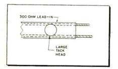
Fig. 1.—How tack head can cause lead-in short.
