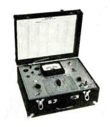
testing of tubes by non-technical clerical help when the checker is used on the counter. Only 5 sockets are used. Tube types are printed on 12-position selector switch; only 2 other controls must be adjusted. Tests for emission, interelectrode shorts or leakage, and gas. Price, \$99.50. Television Engineers, Inc., 311 East 79th Street, Chicago 19, Ill.—TECHNICIAN
