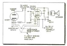
A glance in the tube handbook shows why the 2-tube defect would occur. While the 6W4 has a maximum heater-cathode rating of 450 v when the heater is negative with respect to the cathode, this rating is only 100 v when the heater is positive with respect to the cathode. The 6AQ5, moreover, has a heater-cathode breakdown rating of only 90 volts. Therefore both tubes would break down if the damper tube were defective in this way.
