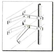
The Y type mount is recommended when greater strength is required for a heavier installation. Rohn Mfg. Co., 116 Limestone, Bellevue, Peoria, Ill.—TECHNICIAN
