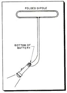
Fig. 5—Checking folded dipole line with flashlight. Bottom cap of flash is first removed.
