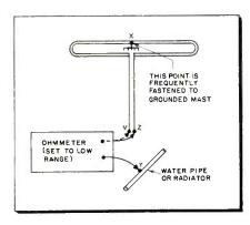
Fig. 4—Testing folded dipole line for continuity. Since point X is electrically the same as Y, sections V-X and Z-X may be effectively checked by testing from V to Y, and Z to Y.
