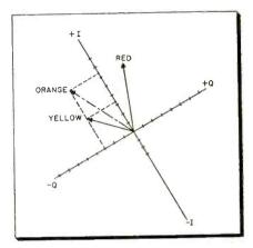
Fig. 2—Effect of doubling 1. Yellow is reproduced as an excessively-bright orange.
