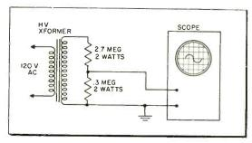
Fig. 1—Test setup for checking industrial-type power transformer. Voltages between 1000 and 5000 v rms (1,400 to 7,000 peak) may be measured with the aid of the voltage-divider shown.
