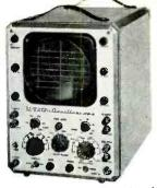
ideal for setting resonant traps, as a general null indicator, signal tracing in low level stages, phase measurements as well as for sweep frequency visual alignment of TV receivers. Has provisions for internal calibration, internal phased sine wave, and Z-axis intensity modulation. Reversal of polarity of both horizontal and vertical signals accomplished by means of toggle switching. Identical vertical and horizontal amplifiers . . . . direct coupling used throughout.
