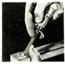
tip of the magnetic core is pushed out flush with the end of the barrel, and magnetically picks up the head of the brad. Then the point of the brad can be directed at any angle desired and inserted in most woods or soft metals by pressure with the palm of the hand. Retail price, \$1.69. Philip Unsinger & Son, 637 Ohio Ave., Fremont, Ohio—TECHNICIAN
