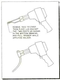
place the lug to be soldered against the two metal posts, as shown, and turn on the switch for a short period, while solder is applied. The method outlined works much faster than one using a simple, old-type iron. The high current drain will not harm the gun over a short period.—
