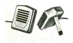
Ceramic model M101 and crystal model M102 hand microphones are compact units housed in plastic cases, designed for prolonged stability. Output of the crystal M102 is —46 db and that of the ceramic M101 is —53 db. Frequency range of the former is 30 to 10,000 cps with flat response, while range of the M101 is 30 to 8000, with slightly rising characteristics in the high range. The M102 lists at \$7.25; the M101 at \$7.00. Astatic Corp., Conneaut, Ohio—TECHNICIAN
