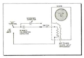
Fig. 2—Sketch illustrating principle underlying capacitance test of an unknown condenser. Deflection on scope screen produced by known capacitor is compared with that of the unknown one.
