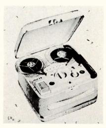
radio as model TR-1000. Hi-fi model T-10 provides response from 60 to 15,000 cps with a tape speed of 7-1/2 in. per sec., ±3 db. Unit features keyboard operation and dual re-
