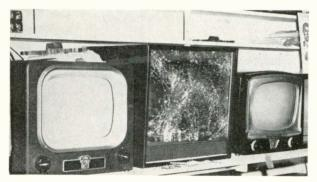
What an implosion can do to safety glass. Controls on front panel have been masked off, in order to prevent identification of the set.
