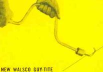
Tighten guy wires faster and better with this new Walsco tool. Does the job of a turnbuckle at a fraction of its cost.
